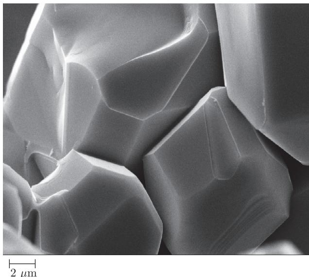
**Fig. 1.** A scanning electron microscopy (SEM) image of the surface of the sample  $(\text{SrFe}_{12}\text{O}_{19})_x(\text{CaCu}_3\text{Ti}_4\text{O}_{12})_{1-x}$
