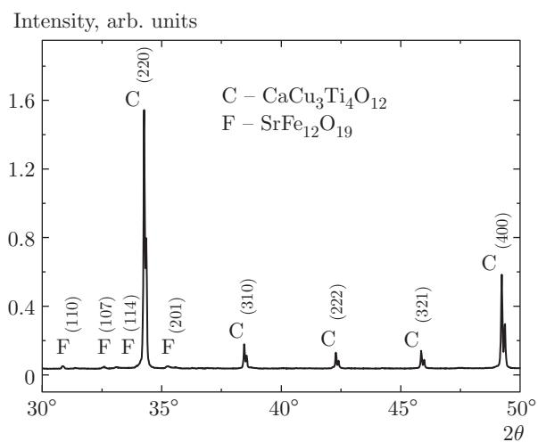
**Fig. 3.** A diffraction pattern  $(\text{SrFe}_{12}\text{O}_{19})_{0.05}(\text{CaCu}_3\text{Ti}_4\text{O}_{12})_{0.95}$  at room temperature
