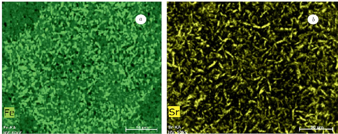
**Fig. 2.** Maps of element distributions in a sample of the  $(\text{SrFe}_{12}\text{O}_{19})_{0.05}(\text{CaCu}_3\text{Ti}_4\text{O}_{12})_{0.95}$  composite: a) Fe, b) Sr (XFA image)**Table 2.** Fitting parameters of the temperature dependence of the  $(\text{SrFe}_{12}\text{O}_{19})_{0.05}(\text{CaCu}_3\text{Ti}_4\text{O}_{12})_{0.95}$  magnetic susceptibility by the Curie–Weiss law
