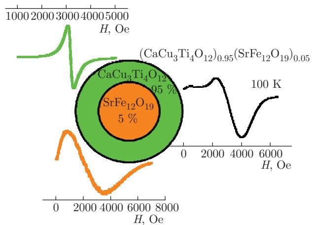
**Fig. 7.** The model “core–shell” of  $(\text{SrFe}_{12}\text{O}_{19})_{0.05}(\text{CaCu}_3\text{Ti}_4\text{O}_{12})_{0.95}$
