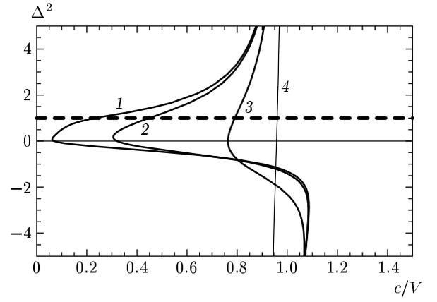
**Fig. 2.** Pulse velocity as a function of the carrier wave frequency for different values of the pulse duration  $\tau$  measured by the parameter  $\Lambda$  (see Eq. (18))  $\Lambda^2 = 0.01$  (1), 0.1 (2), 1 (3), 10 (4)
