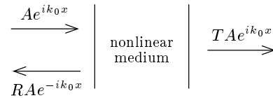
Fig. 2. Reflection and transmission coefficients
