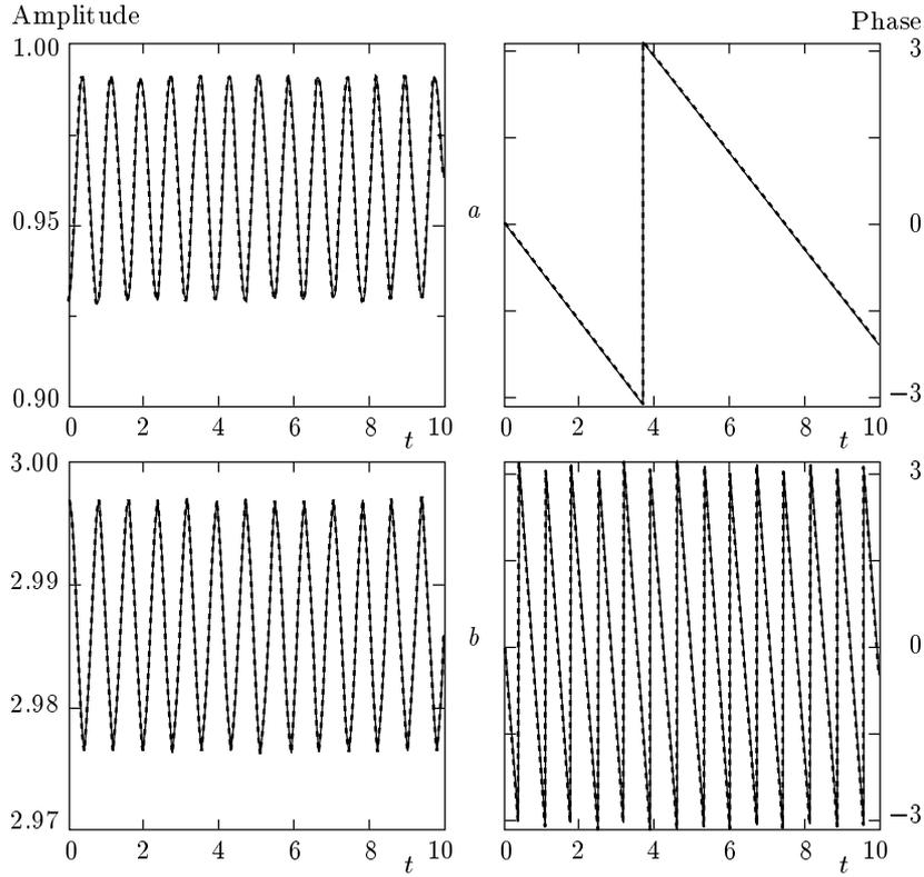
**Fig. 3.** Amplitude oscillations and phase evolution of the excitations in the shock wave transition region: *a)*  $n = -1$ ; *b)*  $n = 1$ ; the parameters are as in Fig. 2. The solid lines show analytical results (3) and the dashed lines correspond to the numerical integration of Eq. (1)
