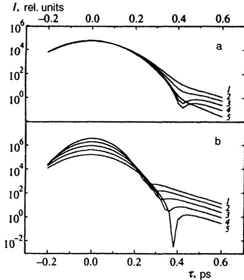
FIG. 4. (a) Shapes of correlation curves calculated for different values of the parameter  $\Delta\omega_{\text{cont}}$ : (1) 30; (2) 33.3; (3) 36.6; (4) 39.9; (5) 43.2 meV ( $t_L=0.11$  ps); (b) for different laser pulse durations  $t_L$ : (1) 0.10; (2) 0.11; (3) 0.12; (4) 0.13; (5) 0.14 ps ( $\Delta\omega_{\text{cont}}=40$  meV). The rest of the parameters used in the calculations are  $T_2^{ba}=4$  ps,  $\Gamma_{hhx}=0.7$  meV,  $T=0.4$  ps,  $\omega_L - \omega_{ba} = -32$  meV.
