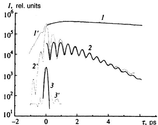
FIG. 3. (1'-3') Experimental and (1-3) theoretical correlation curves for laser pulses whose spectra are given in Fig. 2.
