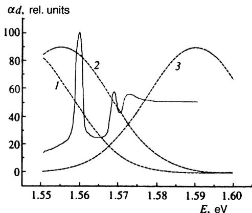
FIG. 2. Absorption spectrum of the sample (solid curve) and spectrum of laser pulses superposed on the exciton spectrum (dashed curves 1-3).
