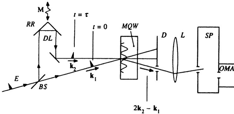
FIG. 1. Diagram of the facility for measuring induced polarization by the four-wave mixing technique.
