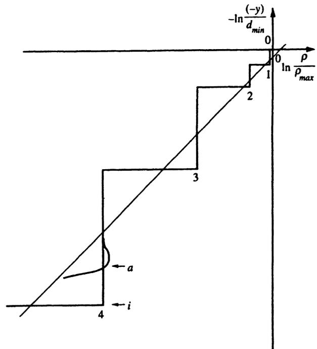
FIG. 4. Stepped distribution of density in a multilayered shell and its continuous approximation.
