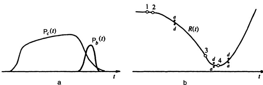
FIG. 2. (a) Power of the compressing pulse,  $P_c(t)$ , and released power  $P_b(t)$ ; (b) radial coordinate  $R(t)$  of the shell driven by the compressing pulse.
