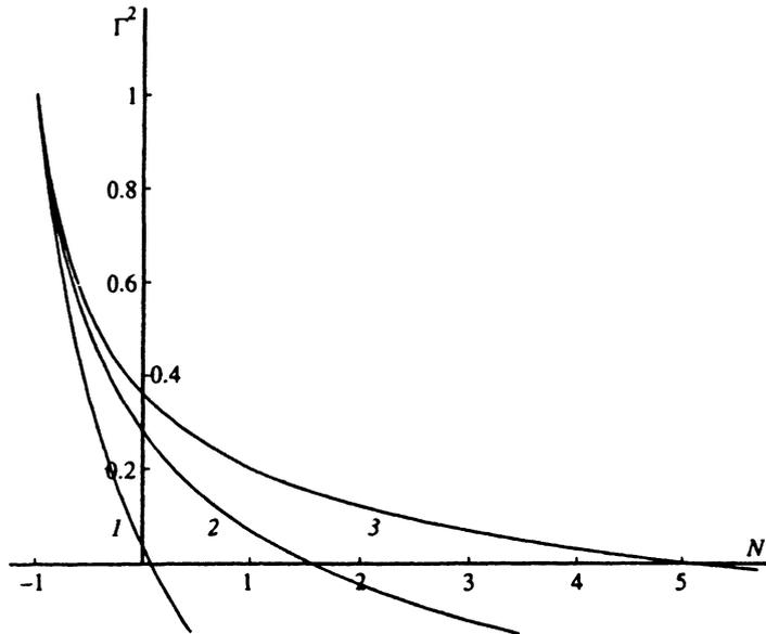
FIG. 5. Damping of instability in profiled shells with masses of the outside layers larger than those of inside layers. In such shells we have  $N > -1$ . The square of the instability growth rate  $\kappa$  divided by the classical limiting growth rate  $\sqrt{gk}$  is plotted against  $N$ . The curves 1, 2, and 3 correspond to the indices  $\gamma = 20$ ,  $5/3$ , and  $1.2$ , respectively. The extreme values of  $\gamma$  are close to those in the incompressible and isothermal cases.
