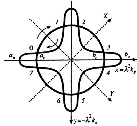
FIG. 1. Trajectories of the valence-band and conduction-band electrons. The centers of the orbits are located at the point  $x=y=0$ . The crossing points of the orbits are numbered (just like the corresponding sectors in the  $\mathbf{k}$  plane; see the Appendix). The arrows indicate the direction of motion of particles in the orbits.
