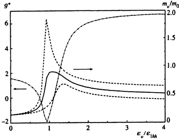
FIG. 2. Dependence of the  $g$  factor (dotted line), the cyclotron mass (solid line), and the maximum and minimum mass in the plane of the well (dashed curves) on the hole energy for the first heavy-hole subband;  $\varepsilon_{1hh} = (\gamma_1 - 2\gamma_2)(\hbar^2 2m_0)(\pi/L)^2$  is the size-quantized energy of the first heavy-hole subband in a well of width  $L$ .
