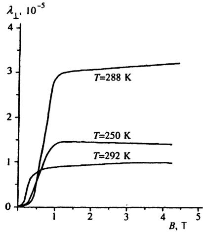
FIG. 3. Field dependence of the transverse magnetostriction of an  $\text{Ni}_2\text{MnGa}$  single crystal in the  $\langle 110 \rangle$  crystallographic direction.
