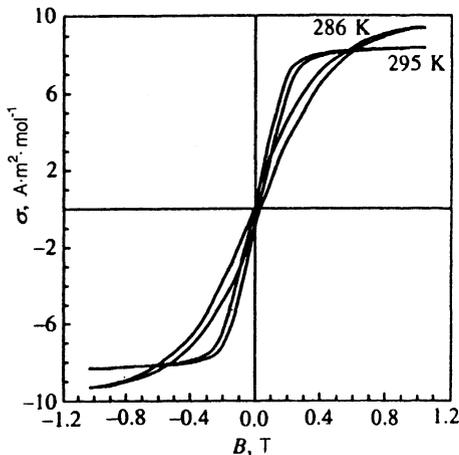
FIG. 2. Field dependence of the magnetization of an  $\text{Ni}_2\text{MnGa}$  single crystal in the  $\langle 110 \rangle$  crystallographic direction near the temperature of the martensitic transformation.
