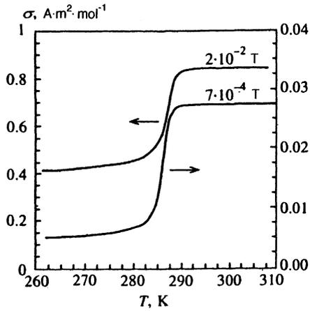
FIG. 1. Temperature dependence of the magnetization of an  $\text{Ni}_2\text{MnGa}$  single crystal in the  $\langle 110 \rangle$  crystallographic direction.
