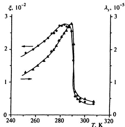
FIG. 4. Temperature dependence of the transverse saturation magnetostriction  $\lambda_s$  and the parameter  $\xi$  of the magnetoelastic coupling in an  $\text{Ni}_2\text{MnGa}$  single crystal in the  $\langle 110 \rangle$  crystallographic direction.
