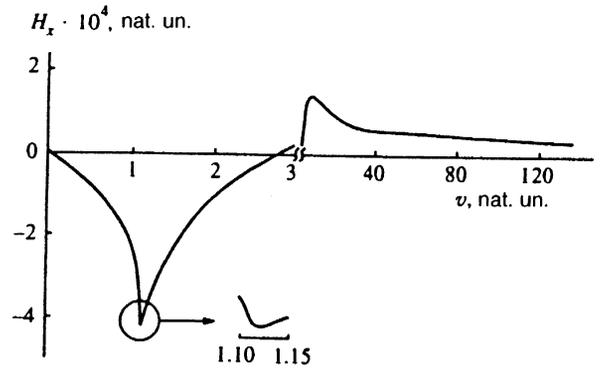
FIG. 3. The polarization magnetic field strength at a proton as a function of the proton's velocity. The proton is moving above an aluminum surface at  $a = 1$  nat.un..
