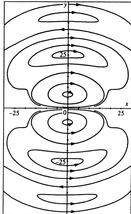
FIG. 1. Magnetic lines of force on the surface of aluminum that are generated as a result of a proton moving with a velocity  $v = 1$  nat.un. ( $v < v_c$ ) at a distance of 1 nat.un. from the surface. The proton is moving in a vacuum along the  $y$  axis above the origin of coordinates.
