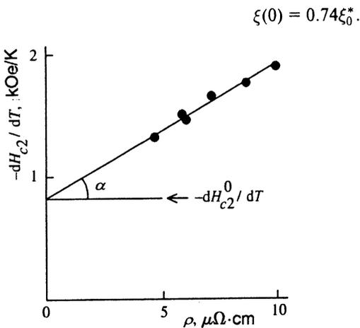
FIG. 2. Dependence of the slope  $-dH_{c2}/dT$  of the temperature dependence of the upper critical magnetic field near  $T_c$  on the resistivity of NbC films.
