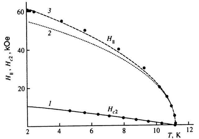
FIG. 3. Temperature dependence of the upper critical field of a thin NbC film with a thickness  $d = 14$  nm in perpendicular ( $H_{c2}$ ) and parallel ( $H_{\parallel}$ ) magnetic fields. The points indicate measured values. 1—plot of  $H_{c2}(T)$  from the GLAG theory; 2—theoretical curve in the Abrikosov model;<sup>19</sup> 3—theoretical curve in the Shapoval model<sup>20</sup> [Eq. (5)].
