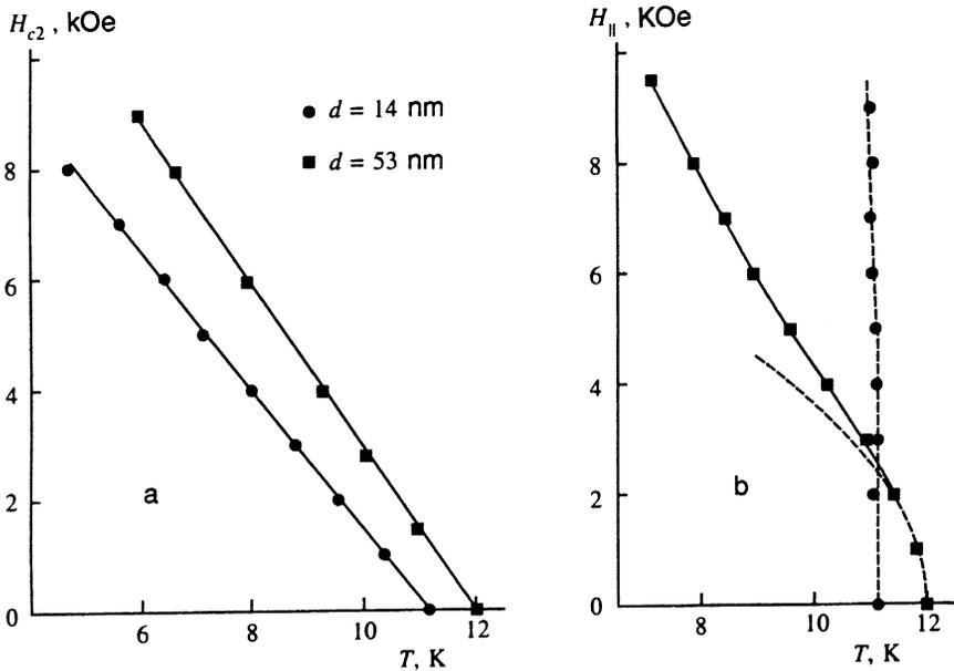
FIG. 1. Temperature dependence of the upper critical field of NbC films of various thickness measured in magnetic fields perpendicular (a) and parallel (b) to their plane. The theoretical curves obtained from Eq. (5) are shown as dashed lines.
