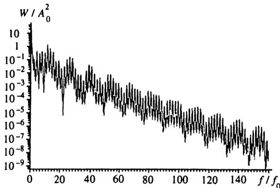
FIG. 4. The spectrum structure over a broad frequency range for a pulse with a Gaussian envelope:  $k = 8$  and  $z = 0.5$ .
