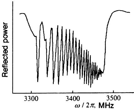
FIG. 1. Typical exchange spin wave spectra in a nonuniform film. The plots show the frequency dependence of the microwave power reflected from the sample, which was a tangentially magnetized YIG film with orientation (111) and thickness  $L=12.5 \mu\text{m}$  in an external magnetic field  $H=563 \text{ Oe}$ .
