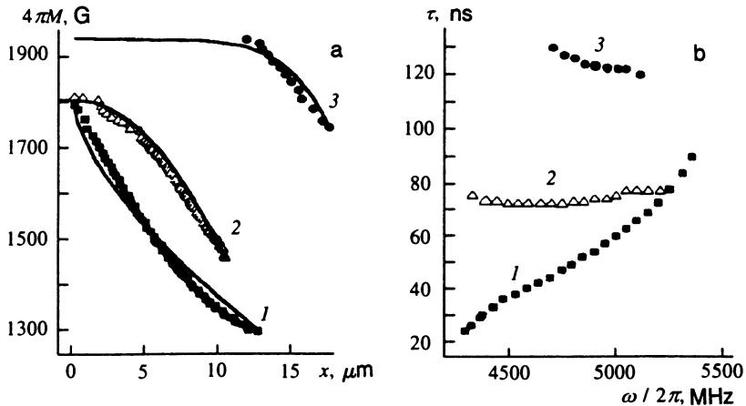
FIG. 7. Profiles of effective magnetization variation (a) for three films with orientation (100) and frequency dependences of the time delay measured on the same films (b). The solid curves 1–3 in Fig. (a) are attempts to approximate the experimental values using power-law functions with exponents  $r=2/3$  (1),  $r=2$  (2), and  $r=6$  (3).
