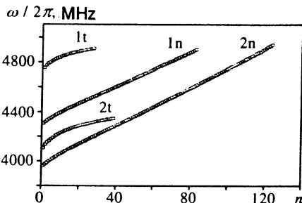
FIG. 2. Dependence of the resonance frequency on mode number. (1t)—sample 1, tangential field  $H=895 \text{ Oe}$ ; (1n)—sample 1, normal field  $H=3588 \text{ Oe}$ ; (2t)—sample 2, tangential field  $H=808 \text{ Oe}$ ; (2n)—sample 2, normal field  $H=3505 \text{ Oe}$  [the YIG films had (111) orientation,  $L=15 \mu\text{m}$  (sample 1) and  $L=17.2 \mu\text{m}$  (sample 2)].
