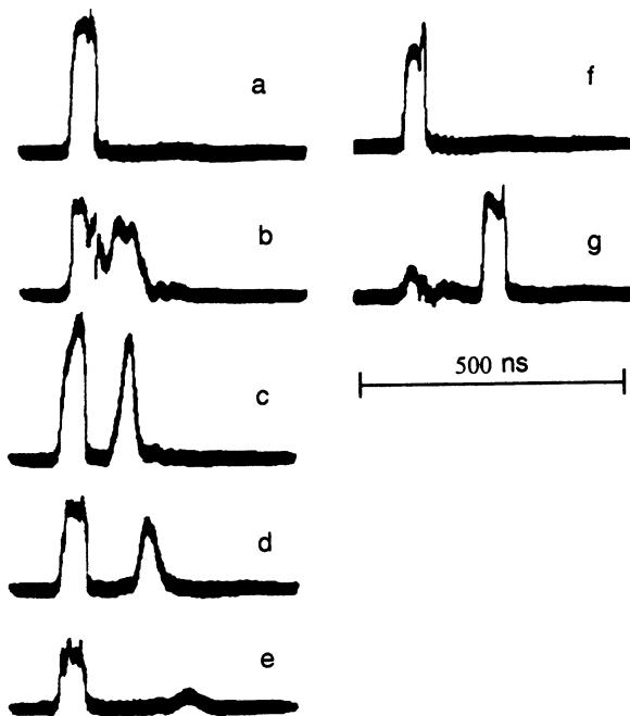
FIG. 5. Time dependences of the envelope of the reflected signal for sample 1. Traces a–e are for a tangential field with  $\omega/2\pi=5124$  MHz; a— $H=0$ ,  $K=0$ ; b— $H=1084$  Oe,  $K=10$  dB; c— $H=1079$  Oe,  $K=10$  dB; d— $H=1071$  Oe,  $K=10$  dB; e— $H=1058$  Oe,  $K=10$  dB. Traces f and g are for a normal field with  $\omega/2\pi=5322$  MHz; f— $H=0$ ,  $K=0$ ; g— $H=3790$  Oe,  $K=7.6$  dB.
