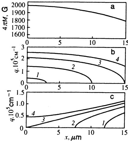
FIG. 3. Profile of magnetization variation (a) and the corresponding computed dependences of the change in wave number versus film thickness for the case of normal (b) and tangential (c) magnetic fields. As an example, we show in (a) a parabolic variation in magnetization. Curves 1–4 in Figs. (b) and (c) reflect the character of the change in wave number for successive increases in frequency.
