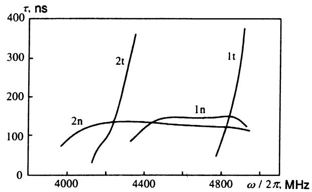
FIG. 6. Dependence of time delay on frequency for samples 1 and 2, computed from the corresponding spectra shown in Fig. 2.
