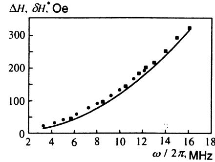
FIG. 11. Computed curve  $\delta H^*(\omega)$  and experimental values of  $\Delta H(\omega)$  for sample 1 (●) and sample 2 (■).
