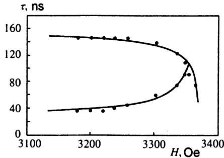
FIG. 15. Dependence of the time delay on magnetic field for sample 1,  $\omega/2\pi=3698$  MHz, normal field. The solid curves are computed values of  $\tau$ , the dots are experiment.
