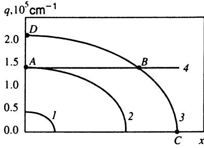
FIG. 10. Variation of the wave number for exchange spin waves along the film thickness. 1— $\delta H < \delta H^*$ ; 2— $\delta H = \delta H^*$ ; 3— $\delta H > \delta H^*$ . Curve 4—wave number for acoustic waves.
