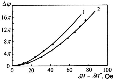
FIG. 13. Dependences of the phase difference on magnetic field. The solid curves are computed values of  $\Delta\varphi(\delta H)$ ; the numbers on the curves correspond to sample number. Experimental values for the first (●) and second (▲) samples are shown for  $\Delta\varphi$  determined using Eq. (20).
