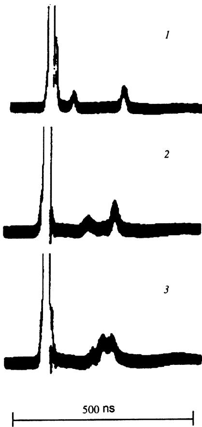
FIG. 14. Time dependence of the envelope of reflected signal for sample 1,  $\omega/2\pi=3695$  MHz, normal field; (1)  $H=2933$  Oe; (2)  $H=3018$  Oe; (3)  $H=3031$  Oe.
