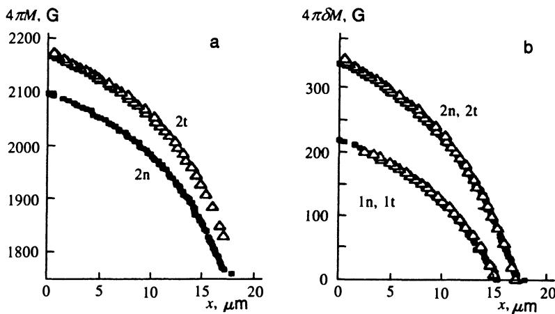
FIG. 4. (a) Profile of effective magnetization variation  $4\pi M(x)$  for sample 2; (b) Profile of relative change of the effective magnetization  $4\pi \delta M(x)$  for samples 1 and 2. These data were obtained by processing the spectra shown in Fig. 2. The points correspond to data calculated from spectra of normally magnetized films, the triangles are from spectra of tangentially magnetized films.
