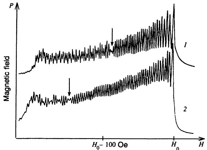
FIG. 9. Dependence of the power absorbed by a YIG film (sample 1) on the magnitude of the external magnetic field for (1)  $\omega/2\pi=7854 \text{ MHz}$ ,  $H_0=4814 \text{ Oe}$ ; (2)  $\omega/2\pi=10300 \text{ MHz}$ ,  $H_0=5587 \text{ Oe}$ .
