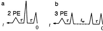
FIG. 1. Optical pulse train resulting in the appearance of two- (a) and three- (b) pulse echo.
