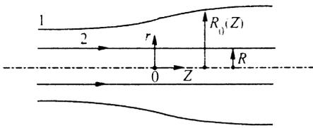
FIG. 1. Model of an open system; 1) waveguide; 2) hollow electron beam.
