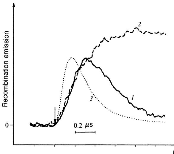
FIG. 8. EHD fluorescence intensity as a function of time elapsed from the excitation pulse (its position is marked by the arrow) for samples of thickness 0.72 mm (1) and 5 mm (2);  $W \approx 120$  erg,  $T = 1.9$  K. Curve 3 is the signal recorded by a photodetector illuminated by the laser pulse.
