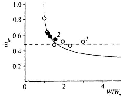
FIG. 6. The results of processing the dependences 1 and 2 presented in Fig. 5 using expression (4). The notation for the dots is the same as in Fig. 5. The solid curve shows the theoretical dependence. The dashed curve shows the transverse sound propagation time.
