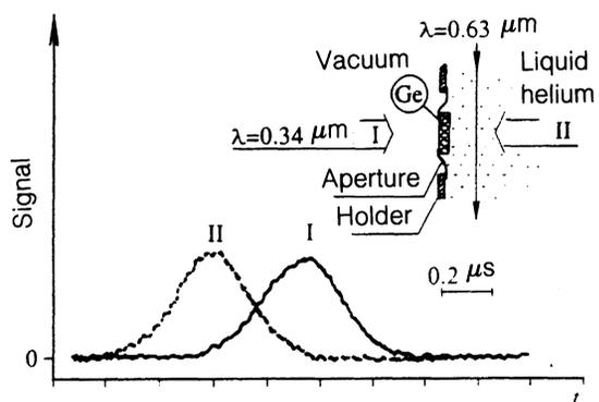
FIG. 2. Signals proportional to the intensity of light diffracted from the pulses of first sound excited in liquid helium at the surface illuminated by laser radiation (II) and at the unilluminated surface (I) of the sample. When recording the pulse I, the pump pulse energy was  $W \approx 120 \text{ erg}$ . The laser spot diameter at the sample was  $\approx 3 \text{ mm}$ . The experimental geometry is shown in the insert.
