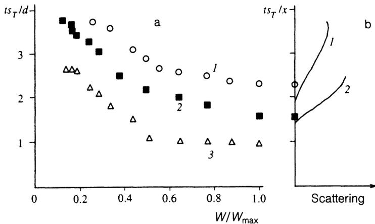
FIG. 7. a) Propagation time of excitations produced with germanium optical pumping through samples of different thicknesses  $d$  as functions of laser pulse energy. 1— $d=0.5$  mm; 2— $d=0.72$  mm; 3—1 mm;  $T=2.1$  K. (b) Kinetics of signal build-up for light scattering from EHDs at different distances [ $x=0.99$  mm (1) and 0.72 mm (2)] from the excited surface (111) of Ge sample 5 mm thick;  $W=W_{max} \approx 120$  erg.
