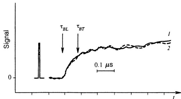
FIG. 9. Kinetics of signal build-up for nonequilibrium phonons detected by bolometer under the conditions of germanium (111) photoexcitation (1) and thermal generator laser heating (2);  $d = 0.72$  mm,  $T = 1.8$  K. The energies absorbed  $W^{abs}$  are the same in both cases. The times of ballistic propagation of longitudinal ( $\tau_{BL}$ ) and transverse ( $\tau_{BT}$ ) acoustic phonons are marked by the arrows. The rectangular pulse shows the position of the pump pulse.
