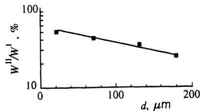
FIG. 4. Ratio  $W^{\text{II}}/W^{\text{I}}$  as a function of sample thickness;  $T=1.7 \text{ K}$ . The slope of the straight line gives the mean free path of nonequilibrium acoustic phonons in resistive processes,  $\Lambda_R \approx 220 \mu\text{m}$ .
