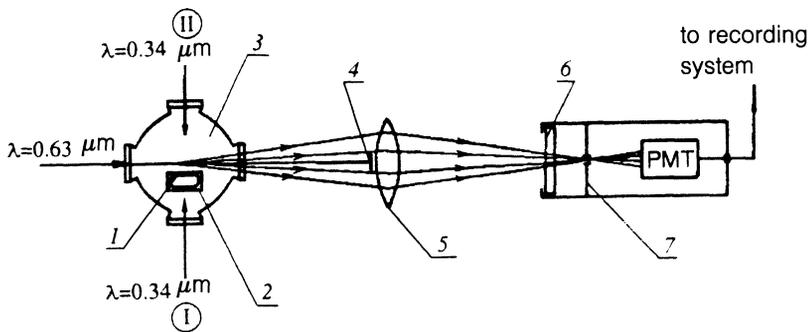
FIG. 1. Optical layout of the experiment. 1) Germanium sample; 2) sample holder; 3) helium bath; 4) beam blocker; 5) collecting lens; 6) filter; 7) entrance aperture.
