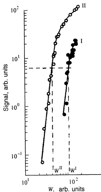
FIG. 3. Signal amplitudes of probing light diffraction from pulses of first sound excited at the illuminated (II) and unilluminated (I) planar facets of a sample of thickness  $130 \mu\text{m}$  as functions of the laser pulse energy;  $T = 1.7 \text{ K}$ .
