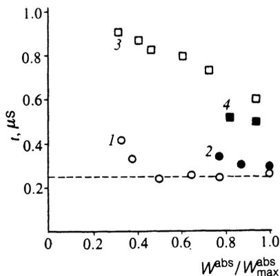
FIG. 5. Excitation propagation time through a sample of thickness  $d=0.72 \text{ mm}$  as a function of the energy absorbed.  $W^{\text{abs}}$  is the maximum energy absorbed by the aluminum film in a single laser pulse. 1,2 Phonons are emitted by the thermal generator; 3,4—excitation of the germanium surface; 1,3— $T=2.15 \text{ K}$ ; 2,4— $T=1.94 \text{ K}$ . The dashed line shows the transverse sound propagation time ( $s_T = 3.07 \cdot 10^5 \text{ cm/s}$ ).
