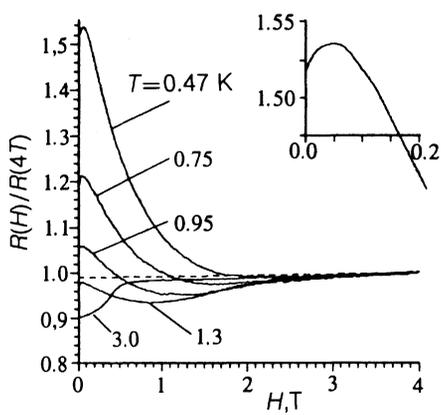
FIG. 3. Magnetic field dependence of the resistance at different temperatures for the state  $q=4.7$ . The dashed line indicates the dependence at  $T=4$  K. Each curve is normalized to the resistance at the given temperature in the field  $H=4$  T. Inset: The part of the curve at  $T=0.47$  K on an enlarged scale.
