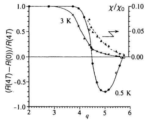
FIG. 4. Relative superconducting response at two temperatures (3 K and 0.5 K) and dynamic susceptibility as a function of the parameter  $q$ . The susceptibility is normalized to the signal corresponding to complete expulsion of the magnetic flux from the volume of the sample; the change occurring in the resistance when a field switched on is normalized to the value of the resistance in the field.
