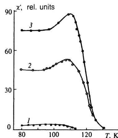
FIG. 3. Differential magnetic susceptibility of  $\text{Bi}_{1-x}\text{La}_x\text{MnO}_3$  for  $x=0.5$  (1),  $x=0.6$  (2), and  $x=0.75$  (3).
