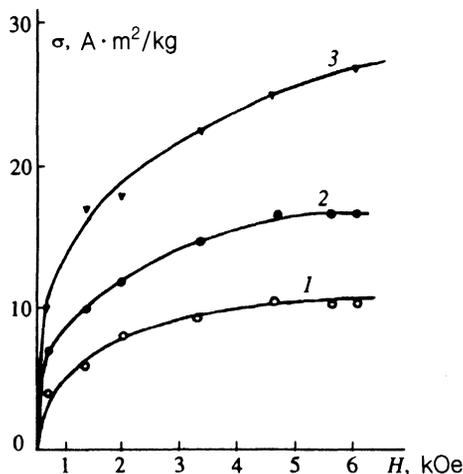
FIG. 4. Field dependence of magnetization for samples of  $\text{Bi}(\text{Mn}_{0.9}\text{Mg}_{0.1})\text{O}_{2.95}$  (1),  $\text{Bi}(\text{Mn}_{0.9}\text{Nb}_{0.1})\text{O}_{3.1}$  (2), and  $\text{Bi}_{0.9}\text{Ca}_{0.1}\text{MnO}_{2.95}$  (3) at  $T=77$  K.
