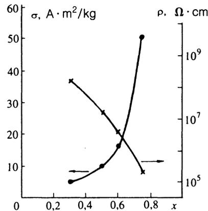
FIG. 2. Dependence of spontaneous magnetization and specific resistivity on composition for the system  $\text{Bi}_{1-x}\text{La}_x\text{MnO}_3$  at  $T=77 \text{ K}$ .
