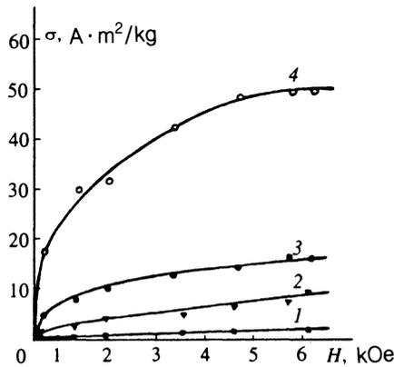
FIG. 1. Dependence of magnetization on field at 77 K for samples of  $\text{Bi}_{1-x}\text{La}_x\text{MnO}_3$  when  $x=0.3$  (1),  $x=0.4$  (2),  $x=0.5$  (3), and  $x=0.75$  (4).
