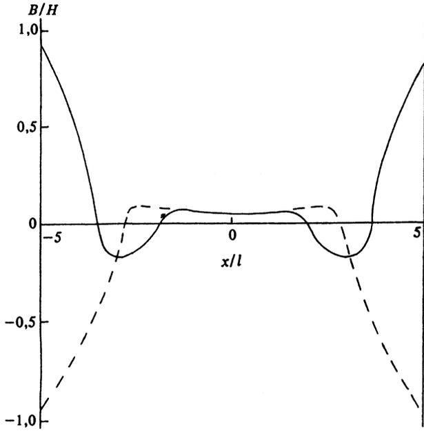
FIG. 10. Distribution of  $B(x,t)$  in a slab of thickness  $L=10l$  at close instants of time:  $\omega t=46$  (solid line), 50 (dashed). The external field  $H \sin \omega t$  is applied at the instant  $t=0$ .
