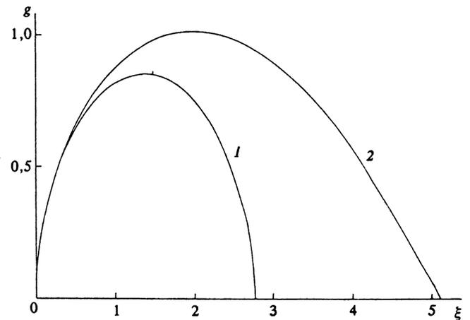
FIG. 2. Scaling functions  $g(\xi)$  describing the evolution of the magnetic flux injected into a superconductor in a zero external field [see (13)]. 1— $\alpha=0$ ,  $\beta=1$ —for a slab. 2— $\alpha=1/4$ ,  $\beta=1/2$ —scaling function for a flux injected into a semi-infinite specimen. The scales of the axes can be consistently changed (see the structure of Eq. (14) for  $g$ ).
