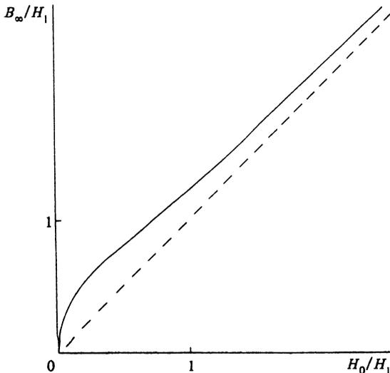
FIG. 5. Dependence of the constant magnetic induction  $B_\infty$  in the interior of a soft superconductor on the value of the constant component of the external magnetic field  $H_a(t) = H_0 + H_1 \sin \omega t$ .
