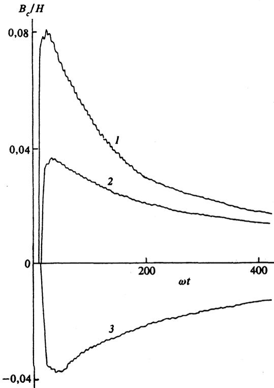
FIG. 11. Time dependence of the magnetic induction  $B_c$  at the center of the slab.  $L=10l$ ,  $t=0$ —instant of application of external field  $H_a=H \sin(\omega t+\varphi)$ ,  $\varphi=0$  (1),  $\varphi=0.4\pi$  (2),  $\varphi=0.6\pi$  (3).
