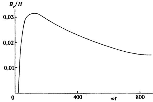
FIG. 12. Dependence of the magnetic induction  $B_c$  at the center of a slab of thickness  $L=15l$  on the time,  $H_a=H \sin \omega t$ .
