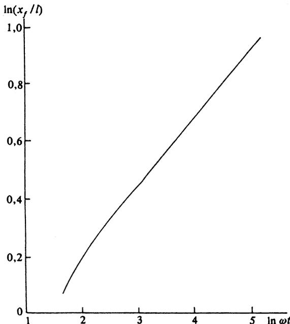
FIG. 9. Plot of the front coordinate vs. time. An external field  $H \sin \omega t$  is applied at the instant  $t=0$ .
