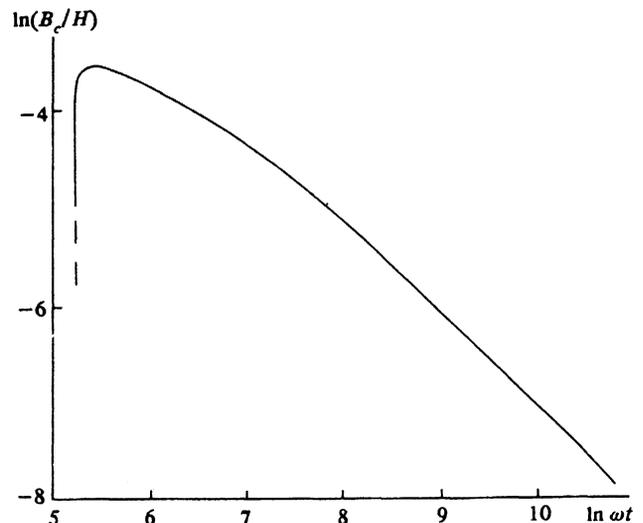
FIG. 13. Dependence of  $\ln B_c$  on the time  $L=15l$ ,  $H_a=H \sin \omega t$ .
