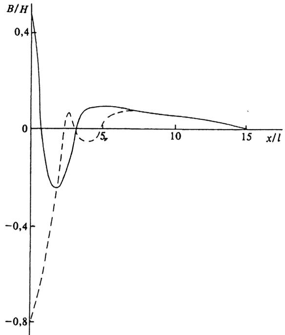
FIG. 7. Coordinate dependence of  $B(x, t)$  in a semi-infinite specimen at the instant  $\omega t = 195.25$  after application of an external field  $H \sin \omega t$  ( $t > 0$ ). The dashed line shows the distribution at a close instant  $\omega t = 192.6$ . The two distributions almost coincide in the interior of the specimen.
