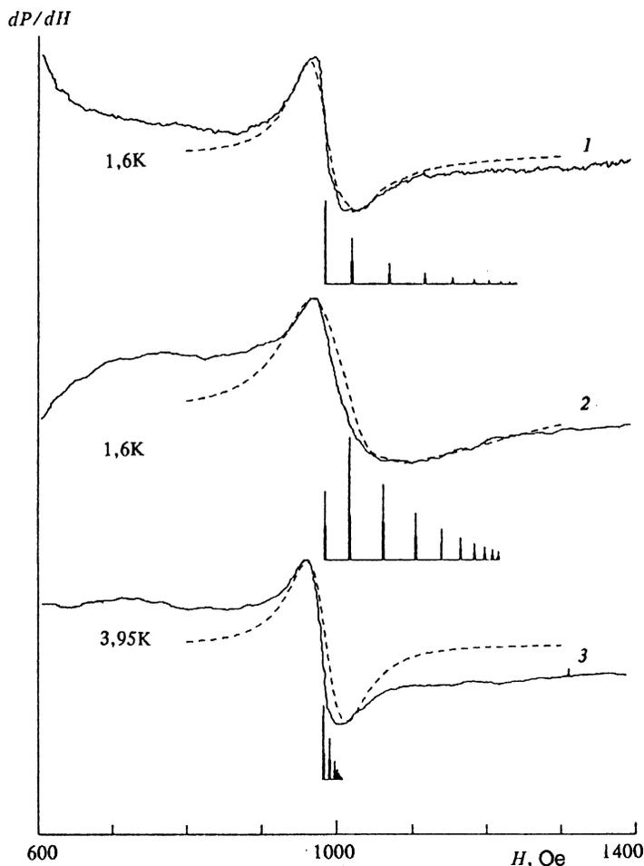
FIG. 3. EPR signal traces for sample N9 at different temperatures with the magnetic field oriented perpendicular (1) and parallel (2 and 3) to the plane of the film. The dashed lines are the computed spectra. The relative intensities and arrangement of the spin-wave resonance lines in the computed spectra are indicated beneath each spectrum.
