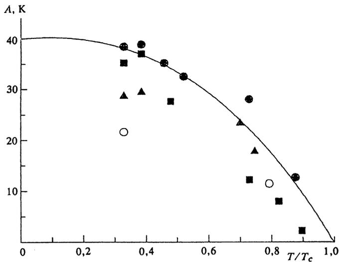
FIG. 5. The parameter  $A$  as a function of the reduced temperature for samples N9 (■), C9 (●), H5 (▲), and C7 (○). The solid line corresponds to  $\delta\chi(T)$  of a BCS superconductor.
