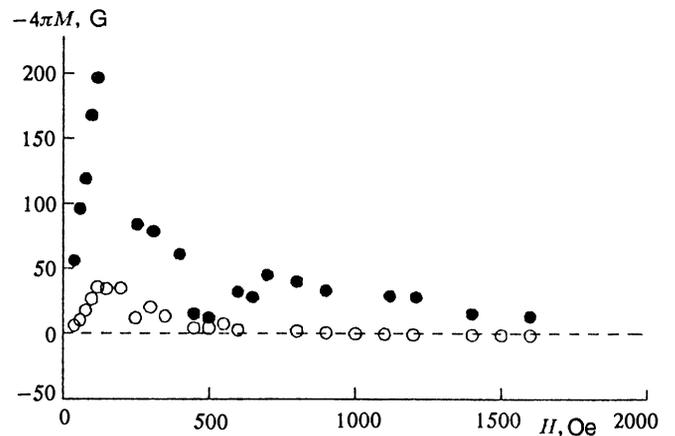
FIG. 2. Magnetization curves for sample H5 with the magnetic field oriented parallel to the sample plane with  $T=4.2$  K (○) and  $T=2.64$  K (●).
