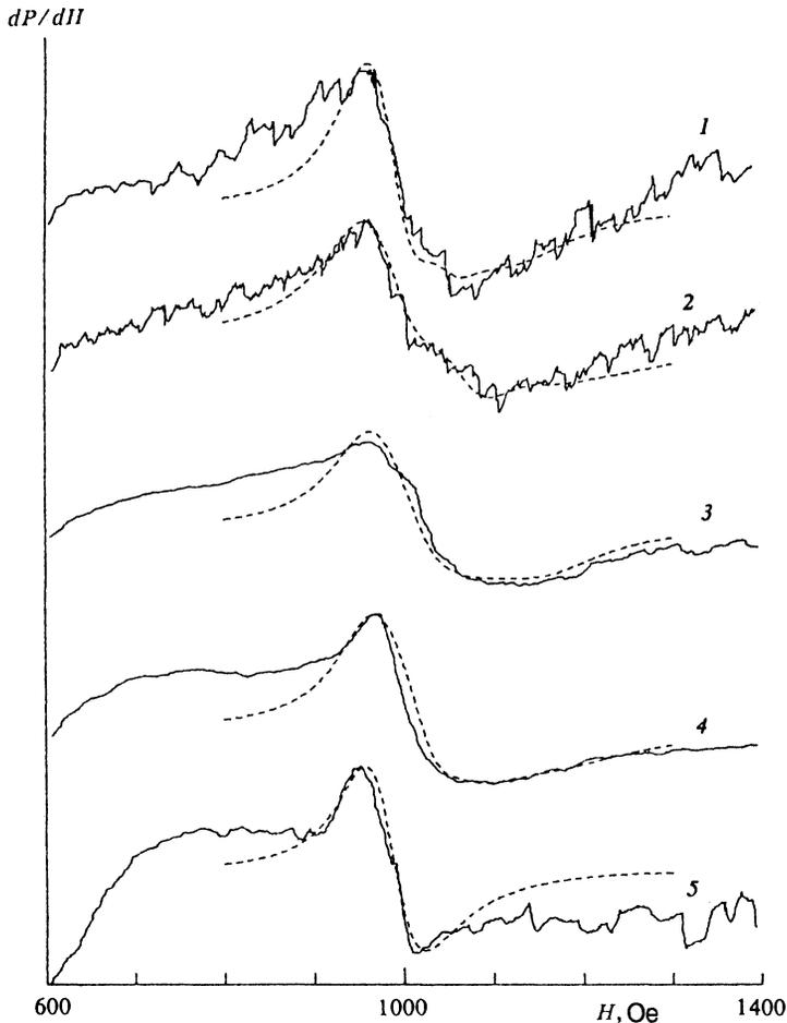
FIG. 4. EPR signal traces for samples C7 (1), H5 (2), C9 (3), N9 (4), H1 (5) at a temperature of 1.6 K with the magnetic field oriented parallel to the surface of the film. The dashed lines were computed.
