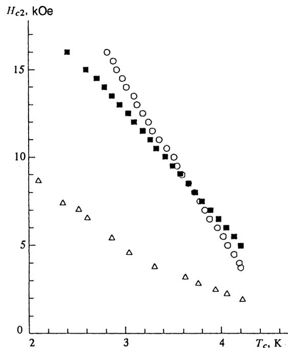
FIG. 1. Temperature dependences of the upper critical field with the magnetic field oriented parallel to the plane of the film for samples H1 (○) and H5 (■).  $\Delta$ —data taken from Ref. 3 for a bulk sample with  $x=0.02$ .
