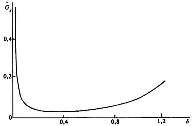
FIG. 2. Theoretical threshold temperature gradient  $G_x$ , normalized to  $q_z^4 \kappa \eta / \rho g \beta$ , i.e.,  $|\bar{G}_x| \equiv G_x \rho g \beta / q_z^4 \kappa \eta$  (see the text proper regarding the notation) as a function of the parameter  $\delta$ , which is the ratio of the sample thickness  $d$  to the effective width of the heated region,  $b$  ( $\delta = d/b$ ).
