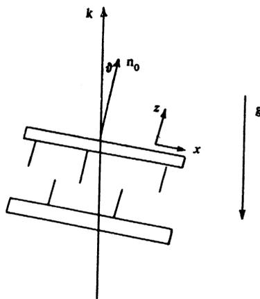
FIG. 1. Experimental geometry.  $n_0$ —Director of the unperturbed nematic liquid crystal (which is along the normal,  $z$ , to the surfaces of the substrates);  $k$ —light wave vector;  $\vartheta$ —angular deviation of the cell from a horizontal position  $g$ —acceleration due to gravity.
