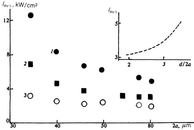
FIG. 5. Experimental threshold intensity  $I_{thr1}$  versus the beam diameter  $2a$  for various sample thicknesses  $d$ : 1—70  $\mu\text{m}$ ; 2—130  $\mu\text{m}$ ; 3—220  $\mu\text{m}$ . Inset: Typical plot of  $I_{thr1}$  versus the parameter  $d$ , the ratio of the sample thickness  $d$  to the beam width  $2a$ , for  $d = 130 \mu\text{m}$  (cf. the curve in Fig. 2 and  $\delta > 1$ ).
