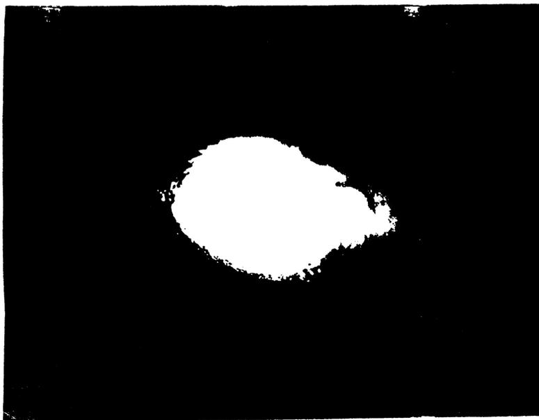
FIG. 6. Diffraction pattern in the case of an oblique orientation of the sample. Scattering "whiskers" can be seen along the direction of the inclination.
