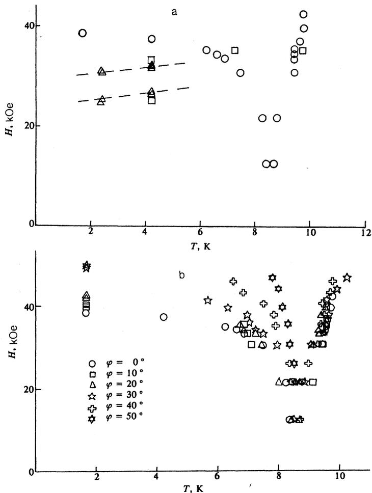
FIG. 3.  $H$  versus  $T$  phase diagram of  $\text{RbMnBr}_3$ , with  $H \perp C_6$  (a) and with different angles between  $H$  and the basal plane (b). In Fig. 3a the circles mark the magnetization breaks, the squares are the data of [9], and the dashed lines correspond to the position of the observed hysteresis of magnetization.
