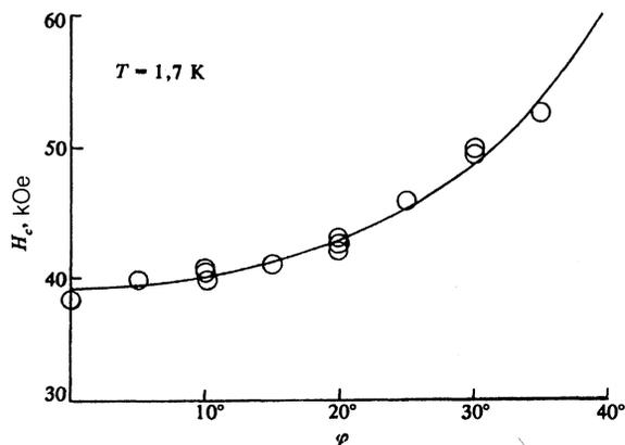
FIG. 4. Critical field  $H_c$  versus the angle between the basal plane and the direction of the magnetic field  $H$ .
