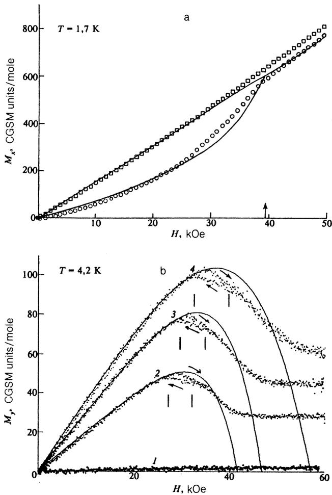
FIG. 1. Magnetizations  $M_x$  (a) and  $M_y$  (b), parallel and perpendicular, respectively, to the magnetic field versus the field  $H$ . The solid lines were calculated using the formulas (3) and (5) for  $M_x$  ( $\square$ — $H \parallel C_6$ ;  $\circ$ — $H \perp C_6$ ) and the formulas of Ref. 2 for  $M_y$ . The data obtained with the field  $H$  making angles of  $0.5^\circ$  (1),  $16^\circ$  (2),  $26^\circ$  (3), and  $36^\circ$  (4) with the basal plane are presented in Fig. 1b.
