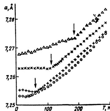
FIG. 8. Temperature dependence of the crystal lattice parameter of several compounds of the system  $(Y_{1-t}Gd_t)(Co_{0.915}Al_{0.085})_2$ ;  $t = 0.03$  ( $\circ$ ),  $0.04$  ( $+$ ),  $0.10$  ( $\times$ ),  $0.20$  ( $\triangle$ ). The arrows show the magnetic ordering temperature.
