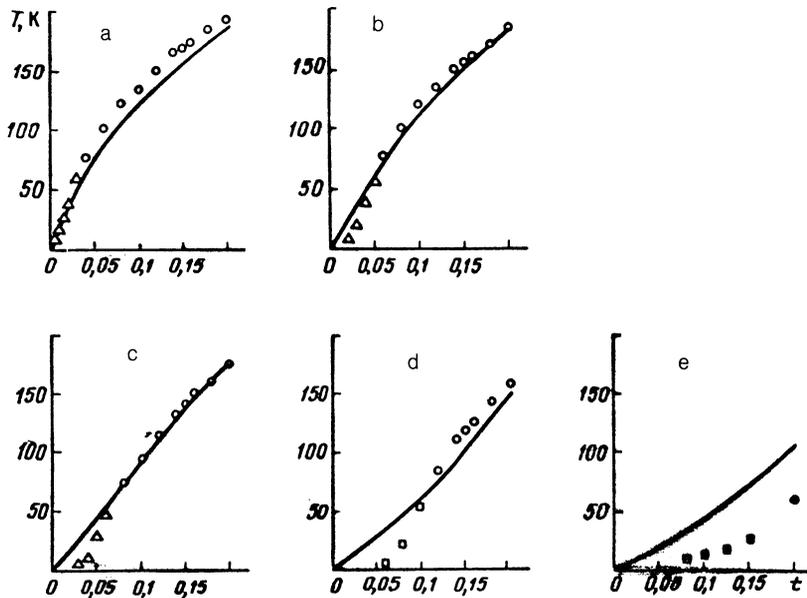
FIG. 7. Magnetic phase transition temperatures of compounds from the system  $(Y_{1-t}Gd_t)(Co_{1-x}Al_x)_2$  as a function of the gadolinium concentration  $t$ .  $\diamond$ —the transition to the strongly ferromagnetic phase,  $\square$ —transition to the weakly ferromagnetic phase,  $\triangle$ —transition to a spin glass state. The curve is calculated theoretically using Eq. (9).
