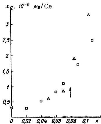
FIG. 5. Dependence of the  $d$ -subsystem susceptibility for the compounds  $Y(\text{Co}_{1-x}\text{Al}_x)_2$  on aluminum concentration  $x$  at 4.2 K using our data ( $\Delta$ ) and the data of Ref. 22 ( $\square$ ). The arrow denotes the critical aluminum concentration at which the magnetization of the rare earth and  $d$ -subsystems become equal, as calculated from Eq. (13).
