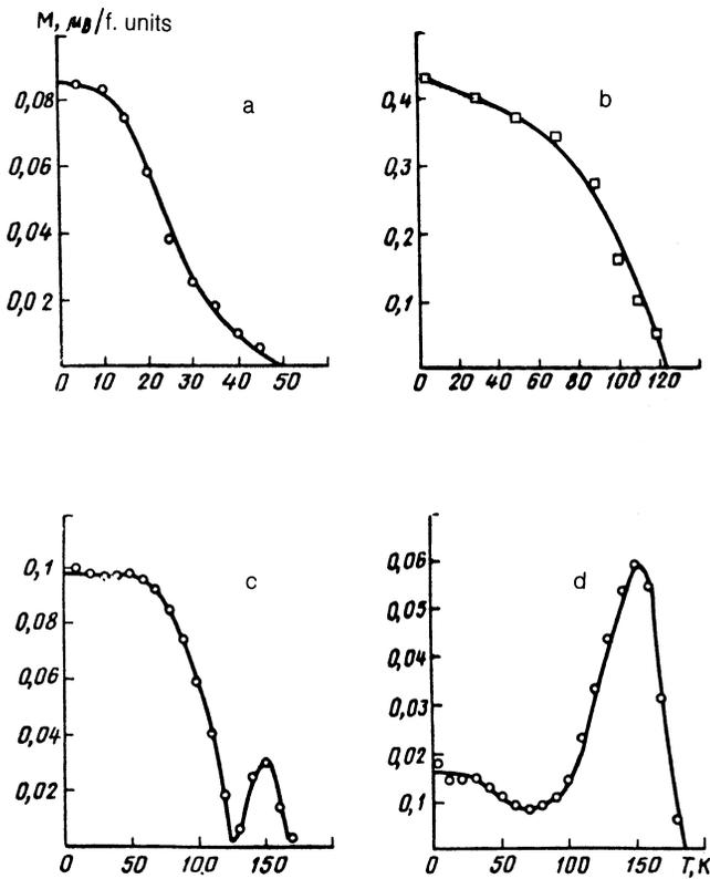
FIG. 9. Temperature dependence of the spontaneous magnetization of several compounds ( $Y_{1-x}Gd_x$ ), ( $Co_{0.915}Al_{0.085}$ )<sub>2</sub>;  $t = 0.04$  (a), 0.10 (b), 0.16 (c), 0.18 (d).
