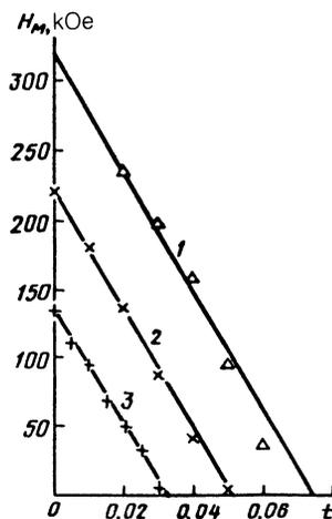
FIG. 4. Dependence of the metamagnetic transition field on gadolinium concentration  $t$  for the system  $(Y_{1-t}Gd_t)(Co_{1-x}Al_x)_2$ ;  $x = 0.07$ , 0.085 (2), 0.105 (3). The straight line is calculated using Eq. (11), and the points are experimental data.
