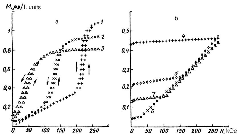
FIG. 2. Magnetization curves of the compounds  $(Y_{1-t}Gd_t)(Co_{0.95}Al_{0.05})_2$  at 4.2 K and  $t = 0.0$  (1), 0.04 (2), 0.1 (3), 0.12 (4), 0.15 (5), 0.18 (6), 0.20 (7).
