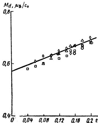
FIG. 6. Magnetic moment of the  $d$ -subsystem for the compounds  $(Y_{1-t}\text{Gd}_t)(\text{Co}_{1-x}\text{Al}_x)_2$  as a function of gadolinium content  $t$  at 4.2 K.  $x = 0.105$  ( $\square$ ),  $0.075$  ( $\diamond$ ),  $0.07$  ( $\times$ ),  $0.05$  ( $\circ$ ).
