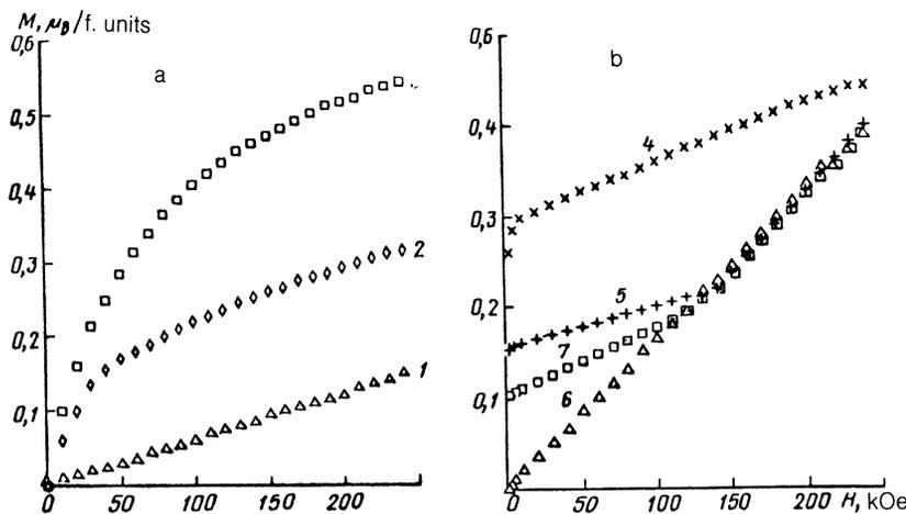
FIG. 1. Magnetization curves for the compounds  $(Y_{1-t}Gd_t)(Co_{0.915}Al_{0.085})_2$  at 4.2 K and  $t = 0.0$  (1), 0.02 (2), 0.04 (3), 0.10 (4), 0.15 (5), 0.18 (6), 0.20 (7).
