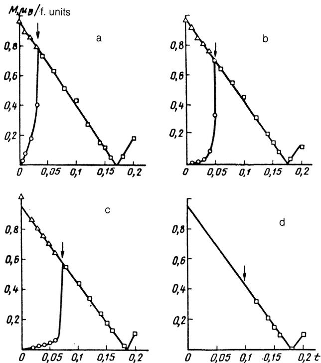
FIG. 3. Dependence of the magnetization on gadolinium content  $t$  for various compounds from the system  $(Y_{1-t}Gd_t)(Co_{1-x}Al_x)_2$  at 4.2 K.  $\circ$ —spontaneous magnetization of the weakly ferrimagnetic compounds,  $\triangle$ —magnetization of the weakly ferrimagnetic compounds in a field of 270 kOe,  $\square$ —spontaneous magnetization of the strongly ferrimagnetic compounds.  $x = 0.105$  (a), 0.075 (b), 0.07 (c), 0.05 (d).
