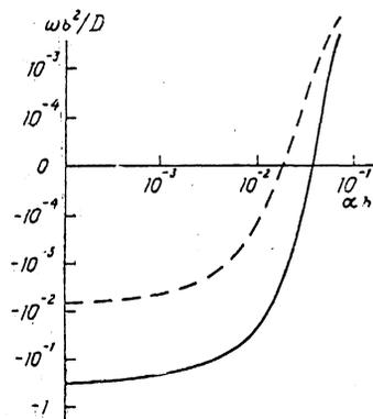
FIG. 2. Growth rate vs dislocation velocity at  $\rho/b = 2$  and  $\lambda/b = 25$ . Solid line— $L/b = -10$ , dashed— $L/b = -5$ .
