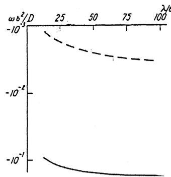
FIG. 3. Growth rate vs wavelength of dislocation line at  $\alpha b = 5 \cdot 10^{-3}$  and  $\rho = 2b$ . Solid line— $L/b = -10$ , dashed— $L/b = -5$ .
