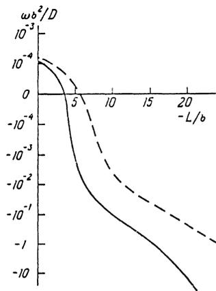
FIG. 1. Growth rate vs intensity of elastic vacancy—dislocation interaction at  $\alpha b = 5 \cdot 10^{-3}$  and  $\lambda/b = 25$ . Solid line— $\rho/b = 2$ , dashed  $\rho/b = 3$ .
