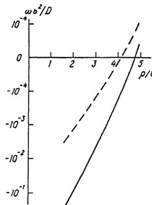
FIG. 4. Growth rate vs dislocation-core radius at  $\alpha b = 5 \cdot 10^{-3}$  and  $\lambda/b = 25$ . Solid line— $L/b = -10$ , dashed— $L/b = -5$ .
