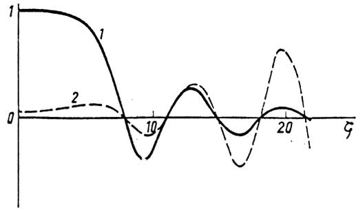
FIG. 3. Shock wave at  $\nu = 0.3$ . 1—The function  $Z(\nu\xi, \xi)$ ; 2—potential at the beam axis,  $\psi(0, \xi)/(20\psi_\infty)$ .
