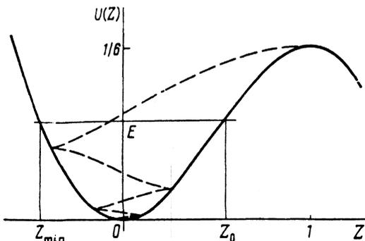
FIG. 1. Plot of the potential energy. The dashed line shows the transformation of a soliton into a shock wave at  $\nu = 0.3$ .
