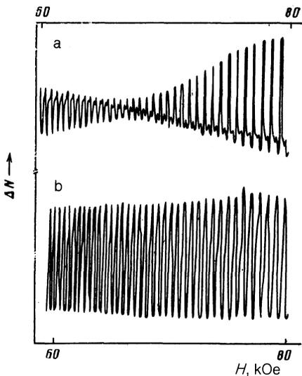
FIG. 4. Magnetic-field dependence of the amplitude of the signal at the piezoelectric transducer detecting the sound. a—Imprecise orientation of the field  $\mathbf{H}$  with respect to the  $[001]$  crystallographic axis; b—with  $\mathbf{H}$  parallel to the  $[001]$  axis as accurately as possible in these experiments.
