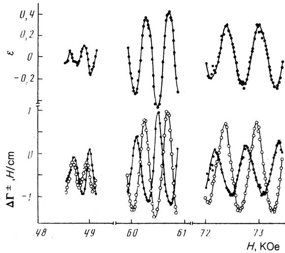
FIG. 1. Absorption of circularly polarized waves and ellipticity of the ultrasound versus the magnetic field. ● — polarization; ○ — + polarization.
