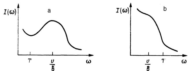
FIG. 3. The spectrum of radiation scattered by a normal metal at low temperatures  $T \ll v/\delta$  (a) and at high temperatures  $T \gg v/\delta$  (b). The typical values of the Fermi velocity  $v \sim 10^8$  cm/s and penetration depth  $\delta \sim 10^{-5}$  cm correspond to the frequency  $v/\delta \sim 50$  cm<sup>-1</sup> ( $1 \text{ cm}^{-1} = 1.44$  K).
