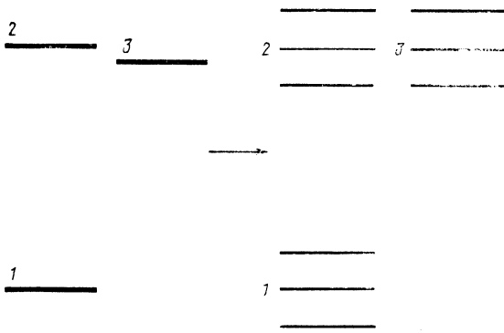
FIG. 3. Diagram of the quasi-energy levels in strong fields. The "intensity" of the middle sublevel of the second level is negligibly small.
