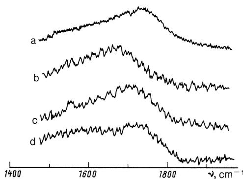
FIG. 3. Comparison of the RS spectra of different modifications of carbon at high pressures: a) a-C (50 GPa), b) single-crystal graphite (50 GPa), c) pyrolytic graphite (50 GPa), d) glassy carbon (44 GPa).
