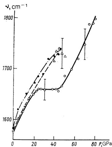
FIG. 2. Pressure dependence of the RS frequencies for (O) single-crystal graphite, (●) glassy carbon, and (Δ) pyrolytic graphite.
