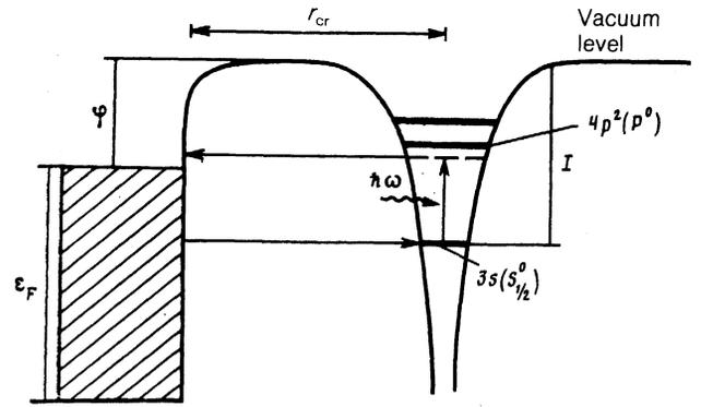
FIG. 1. Diagram of a copper atom evaporated from a copper substrate.
