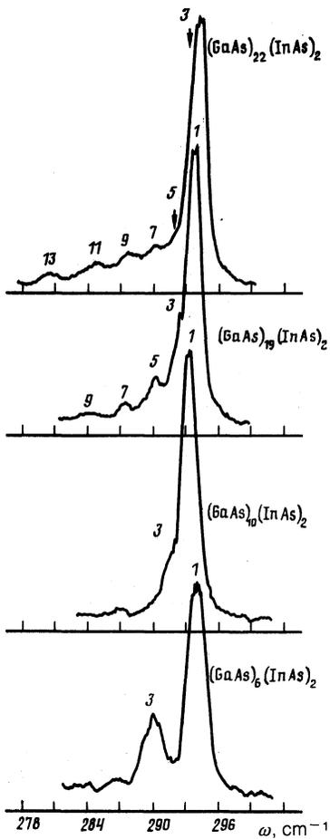
FIG. 5. RS spectra in the optical frequency region of type I SL's;  $xy$  geometry,  $T = 77$  K,  $\lambda_i = 488$  nm.
