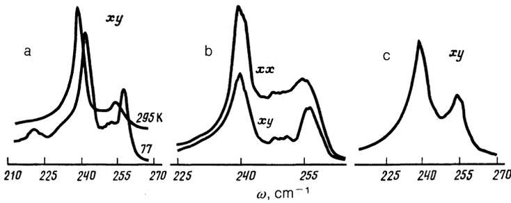
FIG. 8. RS spectra in the optic frequency region a, b) of the SL  $(\text{InAs})_{10}(\text{GaAs})_2$  and c) an aperiodic SL: a— $\lambda_i = 488$  nm; b— $\lambda_i = 476.5$  nm,  $T = 77$  K; c— $\lambda_i = 488$  nm,  $T = 295$  K.
