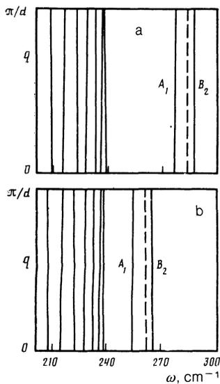
FIG. 9. Theoretical dispersion relation for the SL  $(\text{InAs})_{10}(\text{GaAs})_1$  a) without taking account of mechanical stresses in a GaAs layer and b) taking account of a deformation  $\xi \sim 7\%$  in a GaAs layer. The dashed lines indicate the solutions obtained for the SL  $(\text{InAs})_{10}(\text{GaAs})_1$ .
