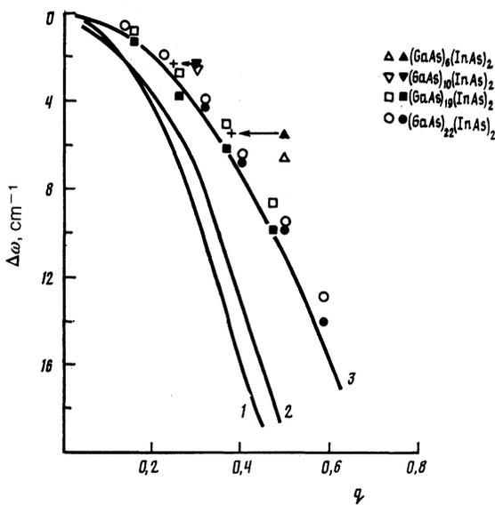
FIG. 6. Theoretical dispersion curves (1,2) of bulk GaAs; 3) a curve constructed from the results of slow neutron scattering in bulk GaAs; the points are experimental (open) and theoretical (dark) values of the frequencies of localized optic phonons in type I SL's.
