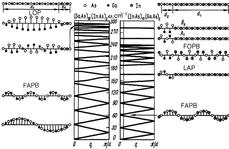
FIG. 2. Theoretical dispersion relations for the SL's  $(\text{GaAs})_{10}(\text{InAs})_2$  and  $(\text{InAs})_{10}(\text{GaAs})_2$ .
