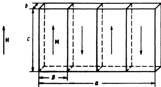
FIG. 1. Structure of the plane-parallel domains.
