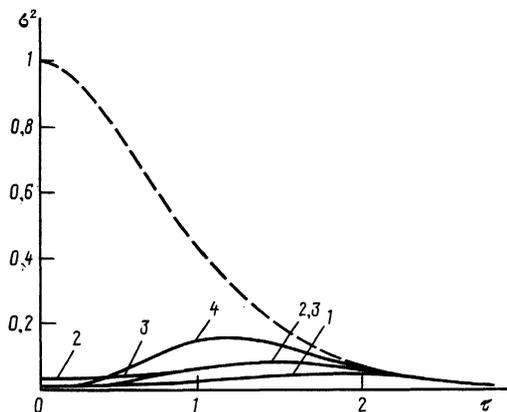
FIG. 4. Plots of the time dependence of normalized dispersion for  $\zeta = 5$ : the dashed curve corresponds to the coherent soliton, curve 1—to optimal amplitude modulation, curve 2—to optimal phase modulation, curves 3 and 4—to mixing with continuous radiation and with a soliton of the same form (there is an error in the labeling of curve 3: for small  $\tau$  it is below curve 2).
