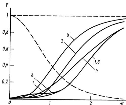
FIG. 3. Plots of the time dependence of the Fano factor for  $\zeta = 5$ : the dashed straight line corresponds to coherent radiation, the dashed curve is the envelope of the fundamental soliton, curve 1 corresponds to optimal amplitude of phase modulation, curve 2—to the approximating phase modulation, curve 3—to the approximating amplitude modulation, curve 4—to mixing with continuous radiation, curve 5—to mixing with a soliton of the same form.
