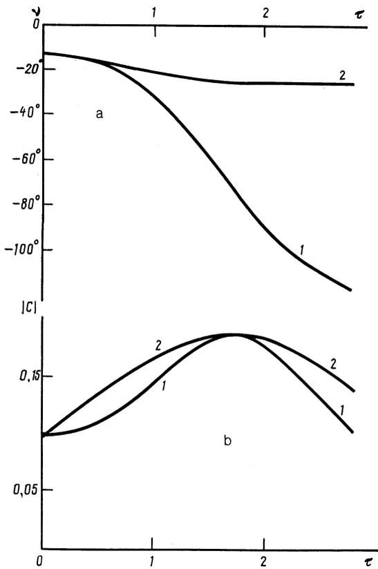
FIG. 2. Plots of the dependence of the phase (a) and the envelope (b) of the auxiliary pulse on the normalized time  $\tau$  for  $\zeta = 5$ ; curve 1 is optimal, curve 2 is approximate.
