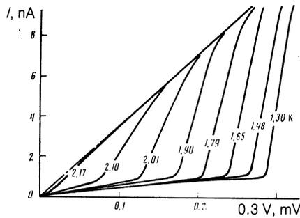
FIG. 1. Current-voltage characteristics at various temperatures (marked on the curve) of a junction with a heat-treated amorphous alloy:  $R = 29 \text{ k}\Omega$ ,  $T_c = 2.18 \text{ K}$ .
