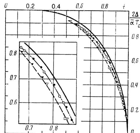
FIG. 3. Superconducting gap as a function of temperature for an amorphous alloy of composition NiZr, alloy quenched (triangles and squares) or heat-treated (circles) alloy. The dark and light symbols pertain to different samples.
