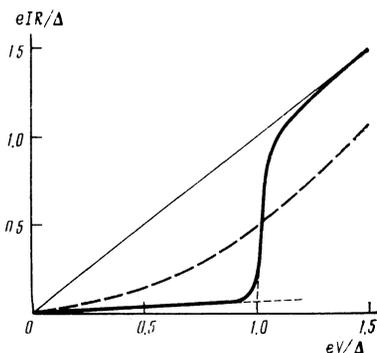
FIG. 2. Comparison of the experimental curve obtained with a non-annealed amorphous alloy at  $T = 1.3 \text{ K}$ ,  $t = T/T_c = 0.53$ , and  $R = 58 \text{ k}\Omega$  (solid curve) with calculation by Eq. (1) for the same  $\Delta$  and  $t$  (dashed line).
