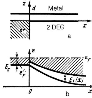
FIG. 2. Model of a contact with a 2DEG in an MIS structure (a, the heavily doped drain or source region is shown shaded) and qualitative behavior of the potential energy of an electron in the 2DEG plane allowing for an inhomogeneity of the channel (b).
