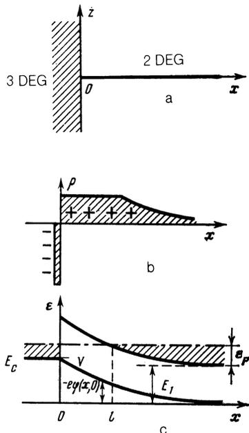
FIG. 1. Schematic representation of a contact between a two-dimensional electron gas (2DEG) and a three-dimensional gas (3DEG) (a), distribution of the surface potential (b), and qualitative behavior of the potential energy of an electron as well as bending of the energy bands in a 2DEG (c). The shaded regions are filled with electrons.
