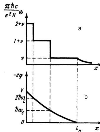
FIG. 3. Distribution of the surface charge along the coordinate in a contact subjected to a strong magnetic field (a) and qualitative behavior of the potential energy of an electron in the 2DEG plane (b).
