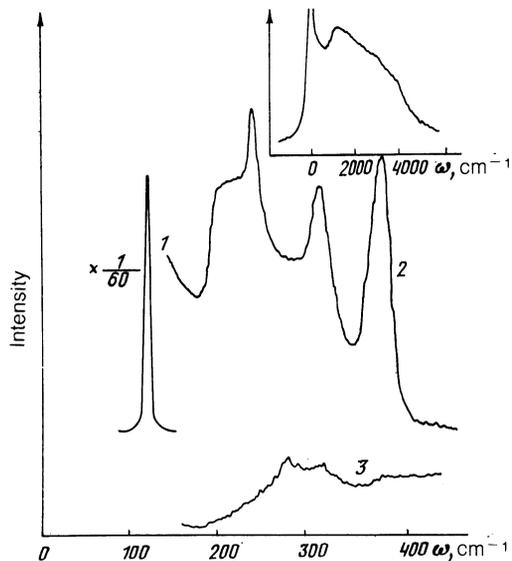
FIG. 1. Spectra of Raman light scattering of first and second orders of a single crystal of rhenium, obtained with a 4880 Å exciting line (2.54 eV) at room temperature: 1—scattering geometry  $YY$  ( $E_{2g}$ ), 2— $YY$  ( $A_{1g} + E_{2g}$ ), 3— $YZ$  ( $E_{1g}$ ). The two-phonon spectrum in the geometry  $YX$  ( $E_{2g}$ ) was not obtained because of the weakness of the signal. Inset—spectrum of rhenium in the region of electron scattering.
