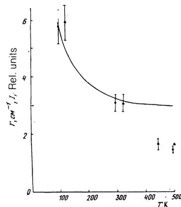
FIG. 3. Temperature dependence of the width of the  $E_{2g}$  line of the phonon (solid curve), intensities of the Raman light scattering spectra of first ( $\bullet$ )<sup>15</sup> and second ( $\blacktriangle$ ) orders in a single crystal of rhenium.
