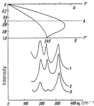
FIG. 4. a—Dispersion of phonons in rhenium along the  $[000 \xi]$  direction,<sup>2</sup> b—two-phonon spectra of Raman light scattering for the  $ZZ$  component of scattering of symmetry  $A_{1g}$  at different temperatures: 1—450 K, 2—330 K, 3—120 K.
