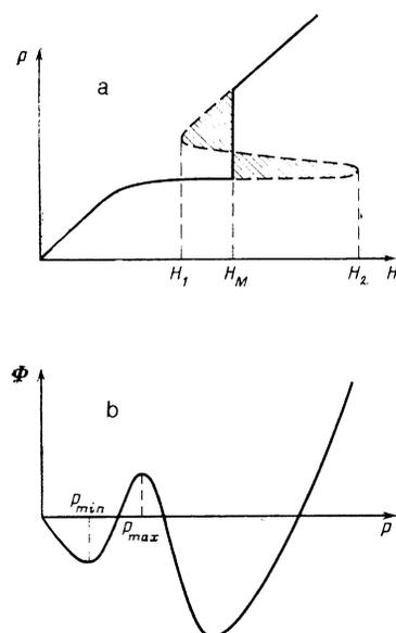
FIG. 1. Schematic representation of the formation of the dependence  $V(H)$  in accordance with the Maxwell principle (a) and the Lyapunov function for the system considered in the range  $H_M < H < H_2$  (b).
