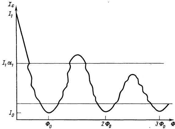
FIG. 2. Dependence of the critical current on the magnetic field in disordered Josephson junctions.
