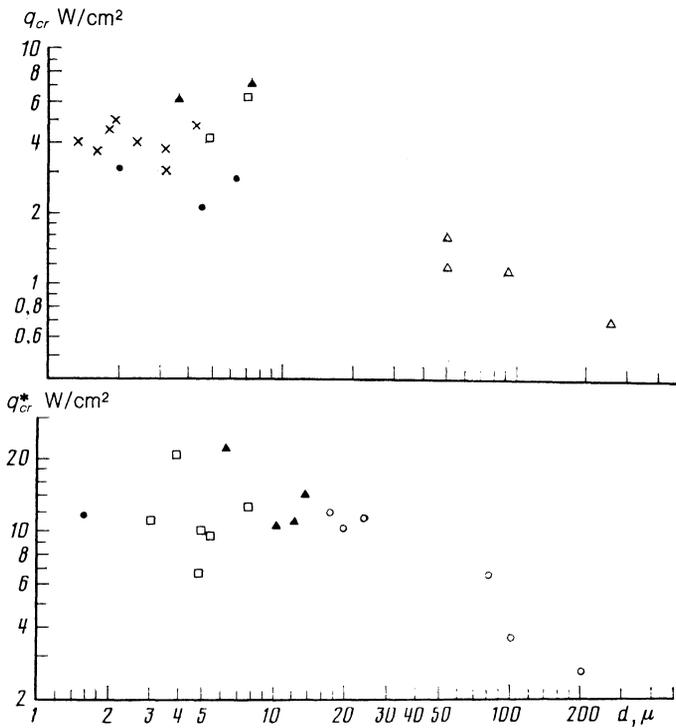
FIG. 1. Dependences of the critical power of the heat flux in liquid helium at 4.2 K ( $q_{cr}$ ) and at 2 K ( $q_{cr}^*$ ) on the thickness of a sample  $d$ : (x) tin whiskers; (□) zinc whiskers; (●) cadmium whiskers; (▲) copper whiskers; (△) Manganin wire (Ref. 10); (○) constantan wire (Ref. 11).
