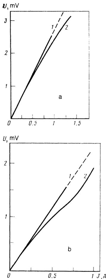
FIG. 2. a) Current-voltage characteristics of zinc whiskers ( $d = 6.6 \mu$ ) at  $T = 2$  K. Curve 1 was obtained before etching, whereas curve 2 was obtained after etching whiskers in HCl vapor. b) Current-voltage characteristics of cadmium whiskers ( $d = 6.2 \mu$ ) at  $T = 2$  K after etching in HCl vapor (curve 2). Curve 1 represents linear extrapolation of the initial part of the characteristic. The voltages  $U$  are given for etched samples.
