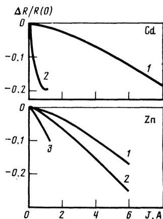
FIG. 3. Dependence of the resistance  $\Delta R/R(0) = [R(0) - R(J)]/R(0)$  of thin samples on the current  $J$ . The upper part of the figure represents cadmium samples: 1) sample of  $0.25 \times 0.12$  mm cross section (Ref. 6); 2) cadmium whisker of thickness  $d = 6.2 \mu$ . The lower part of the figure represents zinc samples: 1), 2) wires with diameters  $d = 0.42$  mm and  $0.23$  mm, respectively (Ref. 2); 3) whisker of diameter  $d = 6.6 \mu$ .
