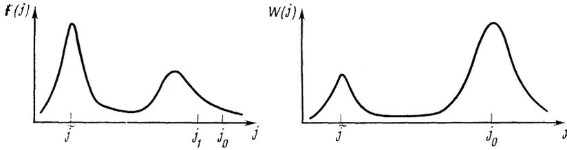
FIG. 1. Probability  $F(j)$  of fluctuations of the critical current density: here,  $j_0$  is the optimal fluctuation in the range of magnetic fields  $|\sin(\pi\Phi/\Phi_0)(\pi\Phi/\Phi_0)^{-1}| \gg \alpha_1$ ;  $j_1$  is the optimal fluctuation in the range of magnetic fields  $\alpha_2 \ll |\sin(\pi\Phi/\Phi_0)/(\pi\Phi/\Phi_0)^{-1}| \ll \alpha_1$ .
