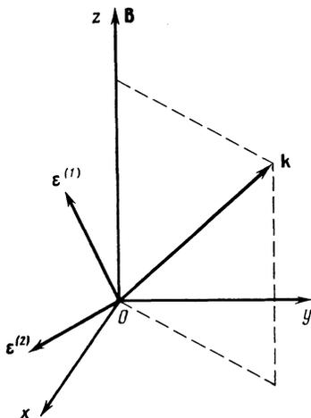
FIG. 2. The photon wave vector  $\mathbf{k}$  and orthogonal linear polarizations  $\boldsymbol{\epsilon}^{(1)}$  and  $\boldsymbol{\epsilon}^{(2)}$  in the selected coordinate system: the vector  $\boldsymbol{\epsilon}^{(1)}$  lies in the plane ( $\mathbf{k}, \mathbf{B}$ ), and the vector  $\boldsymbol{\epsilon}^{(2)}$  is perpendicular to this plane.
