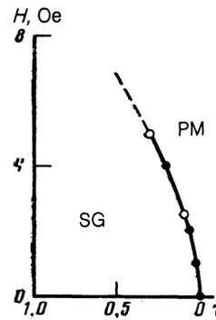
FIG. 5.  $H$ - $T$  phase diagram of the alloy  $\text{Fe}_4\text{Ni}_{76}\text{Cr}_{20}$ .
