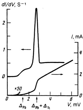
FIG. 1. Current voltage characteristic and first derivative ( $dI/dV$ ) of a Tc/Ta-I-Pb tunnel junction at  $T = 1.6$  K and  $d_{Ta} = 20$  Å. The resistance of the junction in the normal state is  $R_N = 2$  Ω.
