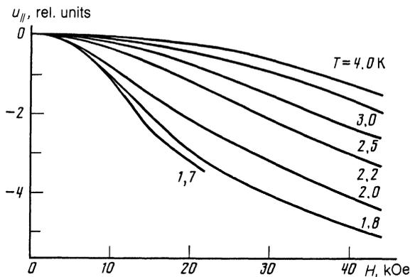
FIG. 4. Isotherms of the longitudinal magnetostriction ( $\mathbf{H} \parallel [011] \parallel \Delta l$ ).
