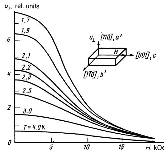
FIG. 3. Isotherms of the transverse magnetostriction of  $\text{TmVO}_4$  ( $\mathbf{H} \parallel [001], \Delta l \parallel [110]$ ) and the measurement geometry. The variation of  $u_1$  with temperature for  $H = 0$  reflects the thermal expansion of the sample.
