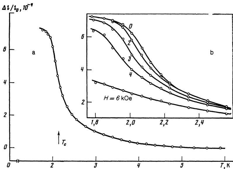
FIG. 1. Thermal expansion of the crystal  $\text{TmVO}_4$  along the  $[110]$  axis for  $H = 0$  (a) and in an external magnetic field  $\mathbf{H} \parallel [001]$  (b).
