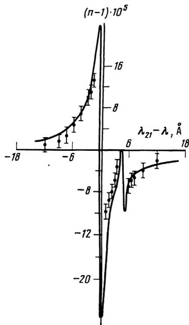
FIG. 3. Dependence of the refractive index on the wavelength (the vertical segments represent the experimental results).
