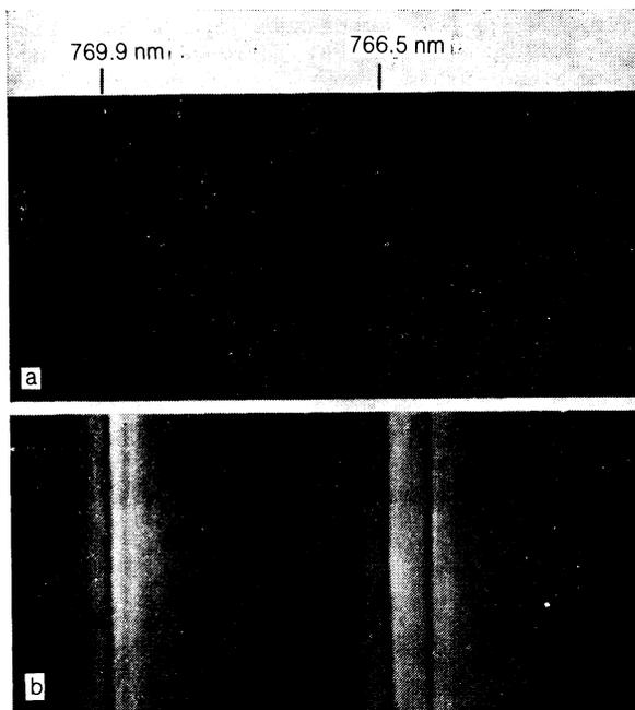
FIG. 4. Emission spectrum of a dye laser with potassium atoms inside the resonator: a) in the absence of ruby laser radiation; b) when ruby laser radiation interacts with potassium atoms.
