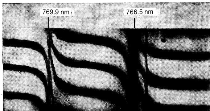
FIG. 2. Interference pattern reflecting the behavior of dispersion near a resonance transition.
