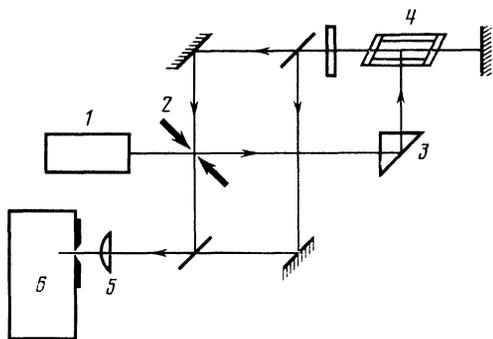
FIG. 1. Schematic diagram of the apparatus: 1) ruby laser; 2) arc discharge; 3) prism; 4) dye cell; 5) cylindrical lens; 6) spectrograph.
