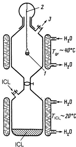
FIG. 1. Apparatus used in the synthesis of iodine monochloride ICG: 1) graphite; 2) quartz spring; 3) vacuum pump.
