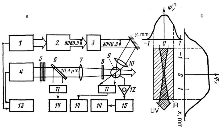
FIG. 1. a) Block diagram of the apparatus: 1—XeCl excimer laser; 2—dye laser; 3—KDP crystal; 4— $CO_2$  laser; 5— $CaF_2$  absorbers; 6— $NaCl$  plate; 7— $NaCl$  lens,  $f = 150 \text{ cm}$ ; 8—cylindrical  $NaCl$  lens,  $f = 12 \text{ cm}$ ; 9—ionization chamber; 10—quartz lens,  $f = 4.5 \text{ cm}$ ; 11—pyroelectric detector; 12—head amplifier; 13—Ch3-34 frequency meter; 14—V4-17 pulse voltmeters; 15—U2-6 amplifier. b) Section through the IR caustic.
