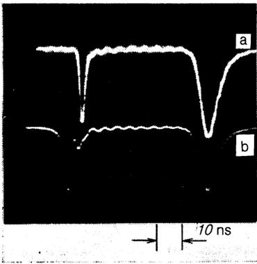
FIG. 1. Time behavior of the radiation intensity at a point in the focal plane at a distance  $r$  from the center of the caustic. The second pulse (incident radiation pulse) is used for time-clamping: a)  $Q = 10^2 Q_{\text{thr}}$ ,  $2\theta = 8 \cdot 10^{-2}$  rad,  $r = 9 \mu\text{m}$ ; b)  $Q = 10^3 Q_{\text{thr}}$ ,  $2\theta = 0.14$  rad,  $r = 0 \mu\text{m}$ .
