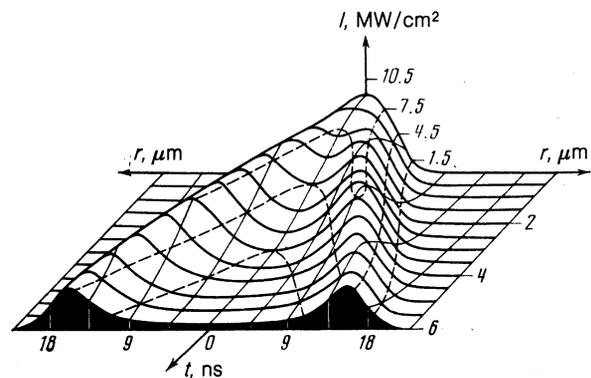
FIG. 2. Intensity distribution in the focal plane as a function of time  $t$  relevant to the instant the intensity at the center of the caustic stopped increasing;  $Q = 10^2 Q_{\text{thr}}$ ,  $2\theta = 8 \cdot 10^{-2}$  rad.
