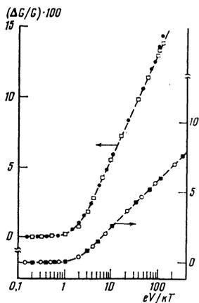
FIG. 3. Dependences of  $\Delta G/G$  on  $eV/kT$  for tunnel contacts in which the disordered electrodes were films Nos. 3 ( $\circ$  and  $\square$ ) and 4 ( $\bullet$  and  $\blacksquare$ ), obtained in  $H = 35$  kOe at various temperatures:  $\circ$ ) 0.4 K;  $\square$ ) 0.6 K;  $\bullet$ ,  $\blacksquare$ ) 4.2 K. The dashed curves are the theoretical dependences represented by Eq. (6).
