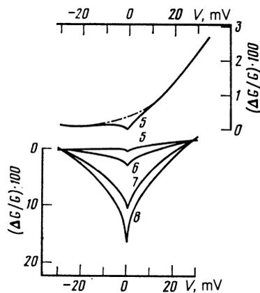
FIG. 6. Dependences  $\Delta G(V)/G$  obtained for tunnel contacts with three-dimensional disordered electrodes at  $T = 0.4 \text{ K}$  in  $H = 35 \text{ kOe}$ . The numbers of the samples are indicated alongside the curves. The dash-dot curve is a parabolic dependence  $\Delta G(V)/G$  observed for pure samples and associated with barrier effects.
