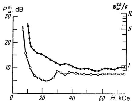
FIG. 6. Dependences of the threshold power  $P_\omega^{\text{th}}$  on the magnetic field  $H$  applied to Bi-2 sample at  $T = 4.2$  K: (●)  $\mathbf{H} \parallel C_3$ ,  $\mathbf{E}_\omega \parallel C_2$ ,  $\mathbf{k} \parallel \mathbf{v}_\omega \parallel C_1$ ; (○)  $\mathbf{H} \parallel C_1$ ,  $\mathbf{E}_\omega \parallel C_3$ ,  $\mathbf{k} \parallel \mathbf{v}_\omega \parallel C_2$ . The right-hand scale applies only to the upper curve.
