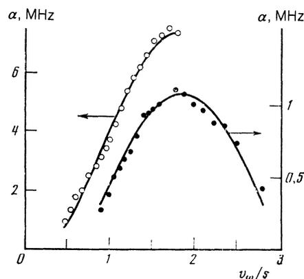
FIG. 4. Dependences of the instability increment on the amplitude of the drift velocity of carriers at  $T = 4.2$  K: (○) Bi-1,  $\mathbf{H} \parallel C_1$ ,  $\mathbf{E}_{\omega} \parallel C_2$ ,  $\mathbf{k} \parallel \mathbf{v}_{\omega} \parallel C_3$ ,  $H = 38$  kOe; (●) Bi-2,  $\mathbf{H} \parallel \mathbf{k} \parallel C_1$ ,  $\mathbf{E}_{\omega} \parallel C_3$ ,  $v_{\omega} \parallel C_2$ ,  $H = 42$  kOe.
