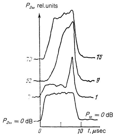
FIG. 2. Profile of the second harmonic pulses generated in sample Bi-2 using different pump powers;  $T = 4.2$  K,  $H = 55$  kOe,  $\mathbf{H} \parallel C_3$ ,  $\mathbf{E}_{\omega} \parallel C_2$ ,  $\mathbf{k} \parallel \mathbf{v}_{\omega} \parallel C_1$ . An increase in the power of the incident wave compared with the power  $P_{\omega}$  for the lower curve is shown on the right and additional attenuation in the receiving channel is shown on the left.
