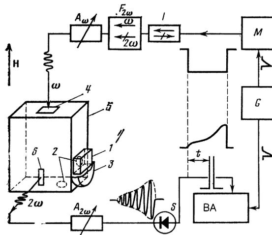
FIG. 1. Schematic diagram of the experimental setup: 1) bismuth sample; 2) apertures; 3) sample holder, acting also as a screen; 4), 6) coupling apertures; 5) resonator;  $A_\omega$  and  $A_{2\omega}$  are attenuators tuned to the frequencies  $\omega$  and  $2\omega$ ;  $F_{2\omega}$  is a second harmonic filter;  $I$  is a ferrite isolator;  $M$  is a magnetron;  $G$  is a synchronization pulse generator;  $S$  is a superheterodyne detector;  $BA$  is a Boxcar-162 analyzer.
