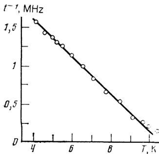
FIG. 5. Temperature dependence of the reciprocal of the growth time of the power  $P_{2\omega}$ : Bi-2,  $\mathbf{H} \parallel \mathbf{k} \parallel C_1$ ,  $\mathbf{E}_\omega \parallel C_3$ ,  $\mathbf{v}_\omega \parallel C_2$ ,  $H = 42$  kOe.
