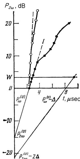
FIG. 3. Time dependences of the power  $P_{2\omega}$  at  $T = 4.2$  K: (○) Bi-1,  $\mathbf{H} \parallel C_1$ ,  $\mathbf{E}_{\omega} \parallel C_2$ ,  $\mathbf{k} \parallel \mathbf{v}_{\omega} \parallel C_3$ ,  $v_{\omega}/s = 1.0$ ,  $H = 38$  kOe; (●) Bi-2,  $\mathbf{H} \parallel \mathbf{k} \parallel C_1$ ,  $\mathbf{E}_{\omega} \parallel C_3$ ,  $v_{\omega} \parallel C_2$ ,  $v_{\omega}/s = 1.3$ ,  $H = 42$  kOe.
