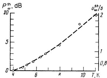
FIG. 7. Temperature dependence of the threshold power  $P_{\omega}^{\text{th}}$ . Bi-2,  $\mathbf{H} \parallel \mathbf{k} \parallel C_1$ ,  $\mathbf{E}_{\omega} \parallel C_3$ ,  $\mathbf{v}_{\omega} \parallel C_2$ ,  $H = 42$  kOe.
