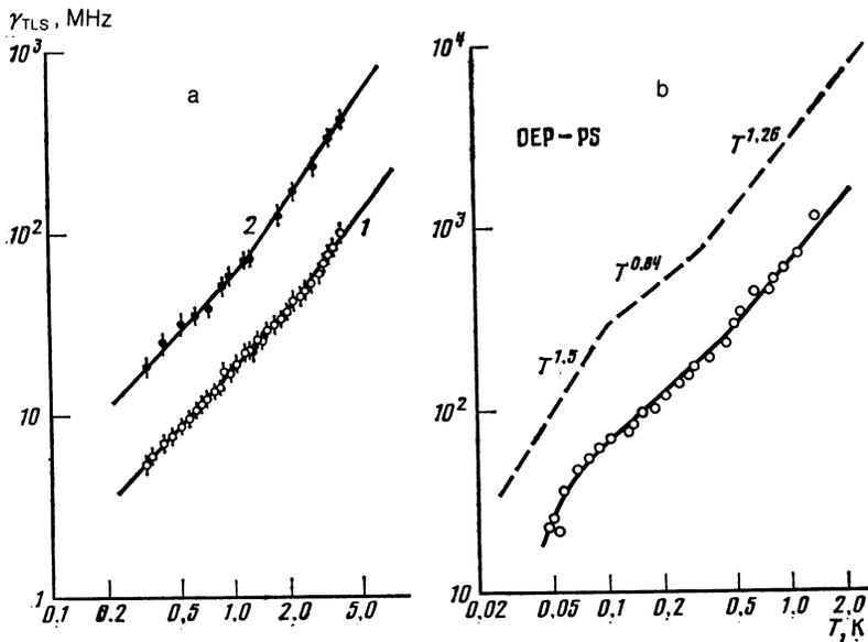
FIG. 2. Comparison of the homogeneous NPL halfwidth measured in Refs. 17 and 19 with the one calculated from Eq. (43) with the function
