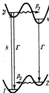
FIG. 1. Adiabatic potentials of impurity center at  $\Delta < 0$ . The transitions 1-3 and 2-4 correspond to resonant and nonresonant fluorescence, respectively.
