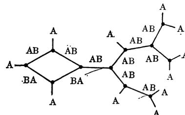
FIG. 5. Branched macromolecule obtained by polycondensation of monomeric units  $\text{RBA}^2$ .
