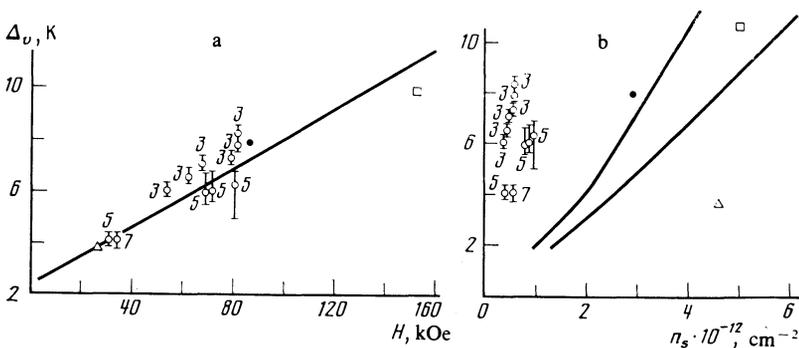
FIG. 5. Valley energy-splitting versus the magnetic field  $H$  (a) and versus the electron density  $n_s$  (b). The numbers labeling the points give the values of  $\nu$ . The points  $\Delta$  and  $\square$  are taken from Ref. 1, Fig. 150; the point  $\bullet$  is from Ref. 17. The solid curves in Fig. b are the theoretical results of Refs. 22 (upper curve) and 23 (lower curve).
