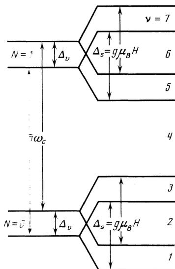
FIG. 1. Energy-level scheme of the *n*-inversion layer in a Si-MOS structure in a quantizing magnetic field.
