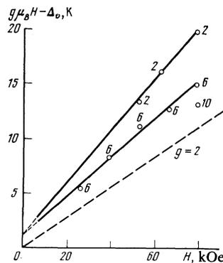
FIG. 8. Values of  $\Delta_\nu$ , for  $\nu = 2, 6, 10$  as a function of the magnetic field  $H$ .
