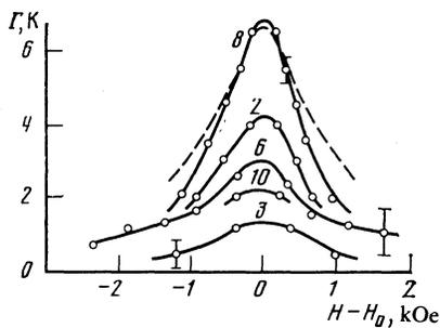
FIG. 6. Level width  $\Gamma$  versus the magnetic field for different  $\nu$  (the numbers labeling the curves);  $H_0 \approx 80$  kOe,  $T = 1.34$  K (for  $\nu = 3$ ,  $T = 0.45$  K). The dashed curve corresponds to the result of Ref. 16 for  $\nu = 4$ .
