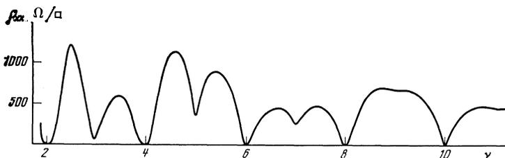
FIG. 7. Resistivity  $\rho_{xx}$  versus the occupation number  $\nu$  of the levels for  $H = 90$  kOe,  $T = 1$  K ( $n_H = 2.16 \cdot 10^{11} \text{ cm}^{-2}$ ).
