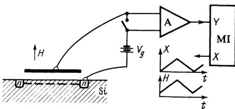
FIG. 2. Schematic of the measurements of the oscillations of the gate voltage: A) amplifier, MI) multichannel integrator.
