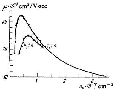
FIG. 3. Mobility of the electrons as a function of their density  $n_s$ .
